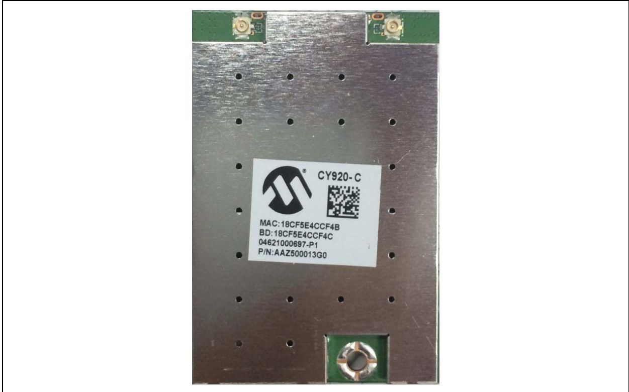
FIGURE 2-3: CY920 BOARD WITH RF SHIELD (TOP VIEW)
