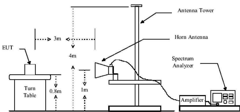
The field strength is calculated by adding the Antenna Factor, Cable Loss & preamplifier. The basic equation with a sample calculation is as follows:
