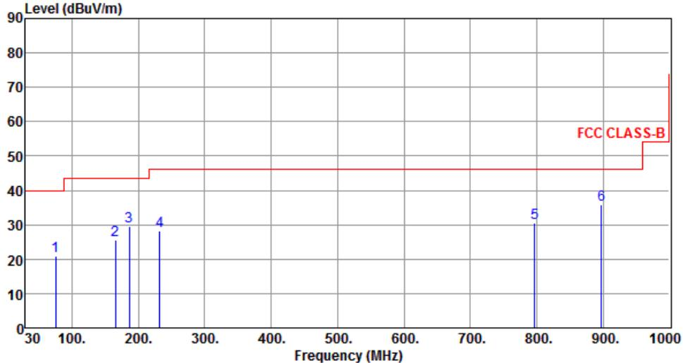
The graph plots Level (dBuV/m) on the y-axis (0 to 90) against Frequency (MHz) on the x-axis (30 to 1000). A red step function represents the FCC CLASS-B limit. Six blue vertical lines indicate emission peaks at frequencies 75.59, 165.80, 186.17, 231.76, 797.27, and 897.18 MHz. The emission levels are 20.90, 25.46, 29.44, 28.36, 30.63, and 35.80 dBuV/m respectively. The limits at these frequencies are 40.00, 43.50, 43.50, 46.00, 46.00, and 46.00 dBuV/m.
