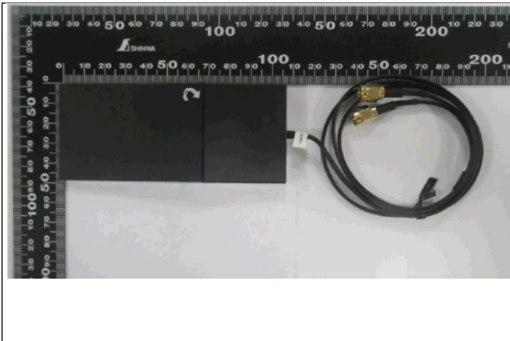
Antenna set 2 (Brand : INPAQ, Model : DAM-I6-H-DB-800-10-17)
