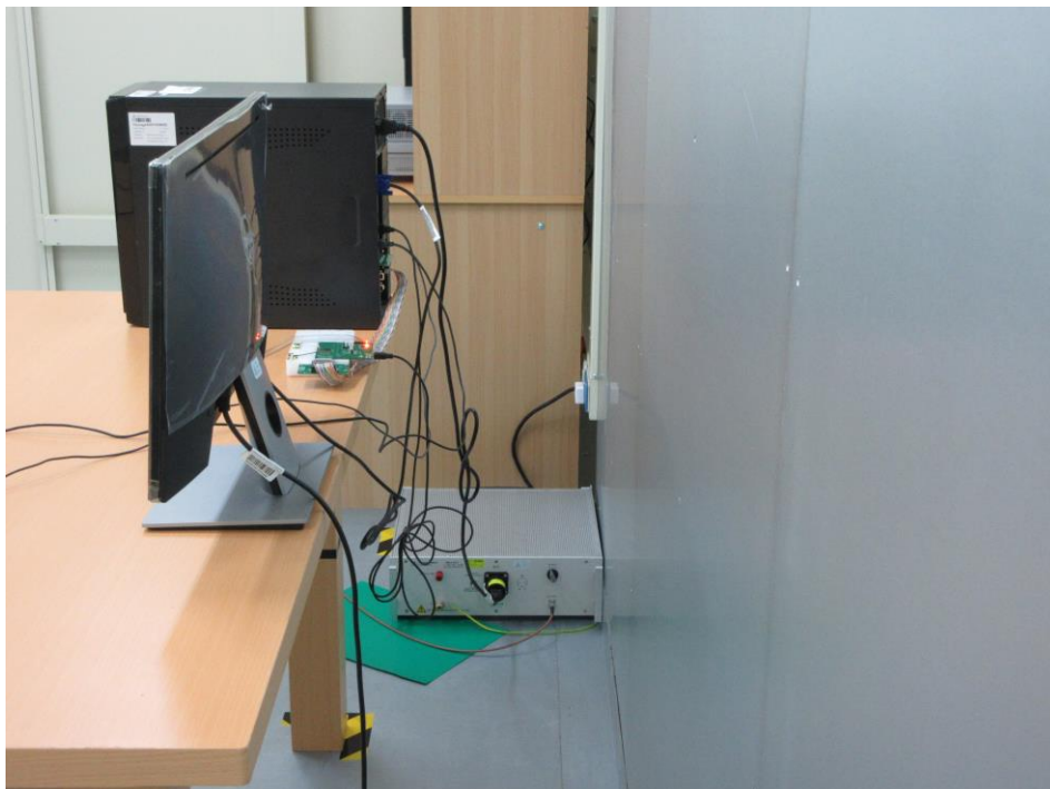
Photograph 8: Set-up for AC Mains (Back View)
