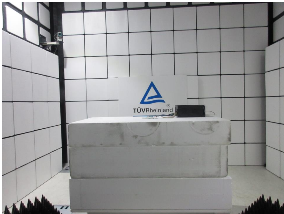
Photograph 2: Set-up for Spurious Emissions (Front View 2)
