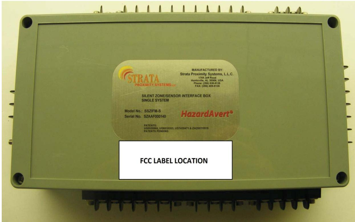
The label is of weatherproof silver polyester as are all of our present labels for harsh environment use. It is laser printer printed and is self stick and supplied on a sheet of 8. It is applied by manufacturing personnel by peeling from the sheet of 8 and pressing on the Surface Proximity Module at the same the module identification label is applied.
