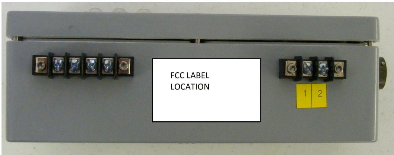
The label is of weatherproof silver polyester as are all of our present labels for harsh environment use. It is laser printer printed and is self stick and supplied on a sheet of 8. It is applied by manufacturing personnel by peeling from the sheet of 8 and pressing on the Surface Proximity Module at the same the module identification label is applied.
