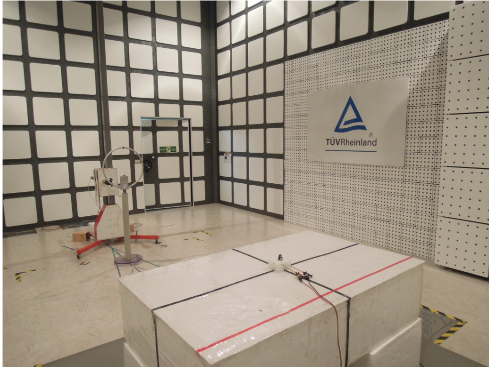
Photograph 6: Set-up for Spurious Emissions (Back View 4)
