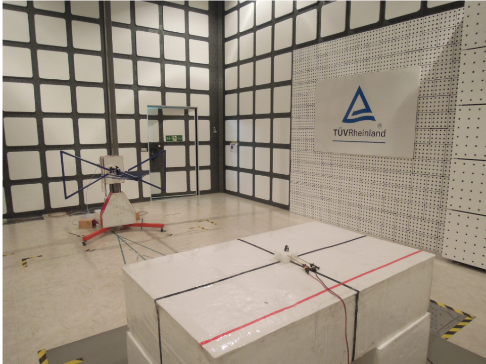
Photograph 4: Set-up for Spurious Emissions (Back View 2)
