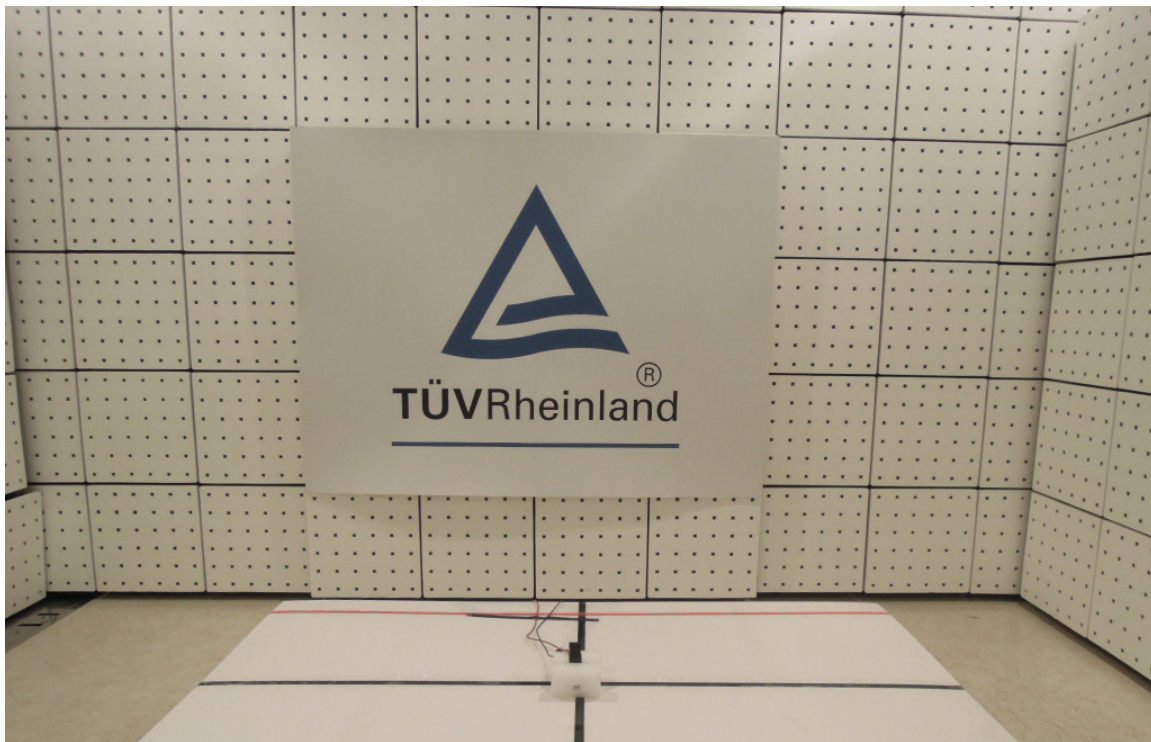
Photograph 1: Set-up for Spurious Emissions (Front View 1)
