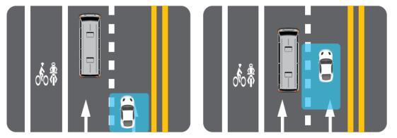
• If the blind spot indicator on the left A-pillar lights up or flashing, it indicates that there is a vehicle entering the left side of your vehicle or a vehicle approaching from the rear left side at high speed. Please slow down and
