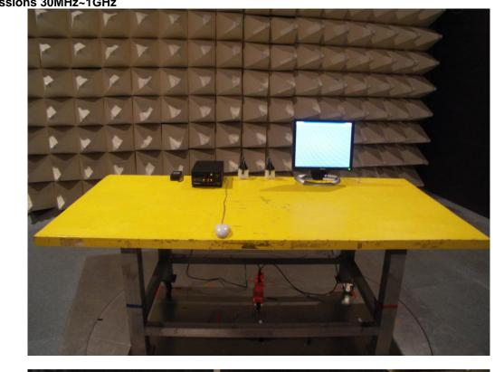
For radiated emissions 30MHz~1GHz
