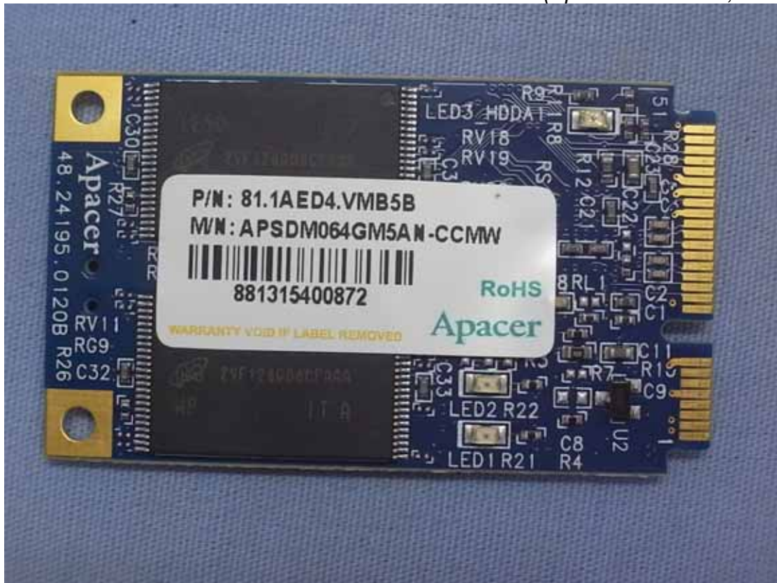
Internal View (Apacer SSD Card, Front View)
