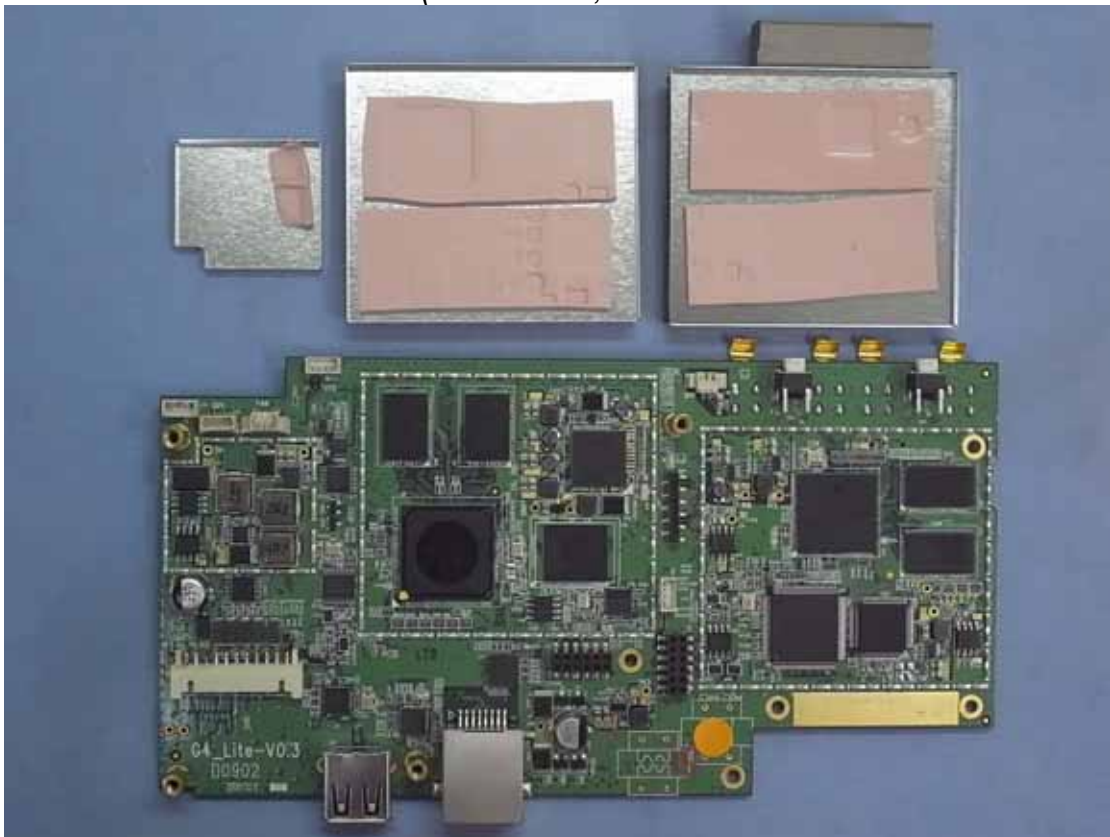
Internal View (Main Board, Front View With Removed Shielded Cover)
