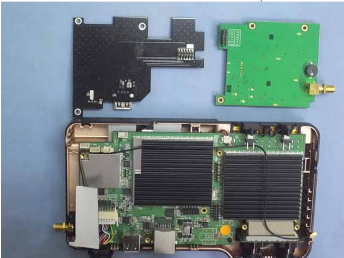
Photo 14 Internal View (Removed Internal Boards)
