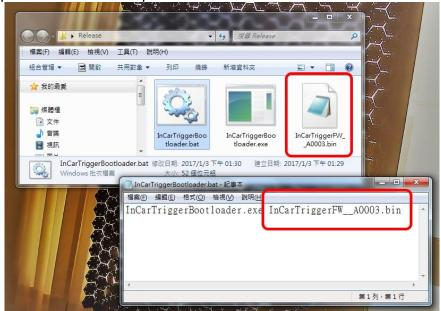
Save and execute InCarTriggerBootloader.bat script to initiate the firmware flushing process and pop up command line window below to notify user the progress of whole process:
