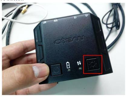
Press the Covert button will switch In-Car Trigger in/out of LEDs covert mode. When In-Car Trigger is in LEDs covert mode, all LEDs will be force turned off regardless the LED notification defined in previous chapters.
