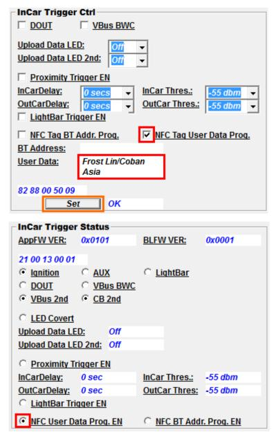
Approach the BWC NFC tag to the sensing area of the NFC reader on In-Car Trigger fixture like section 7.2. The buzzer on fixture would generate 3 short beeps to notify programming complete.
