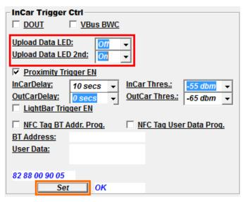
Also, current configuration of Upload data status LEDs would be periodically updated in In-Car Trigger status window.
