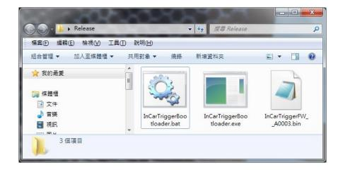
Before launching the firmware flushing process, edit the provided InCarTriggerBootloader.bat script to make sure the filename specified in batch script is identical to the provided \*.bin file.
