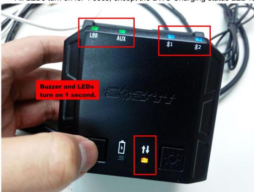
After the notification, buzzer would stop beeping and together with all LEDs start to be controlled based on defined scenario.
