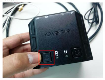
Press the power button will power on/shutdown the In-Car Trigger. refer to chapter 4 about the power on initialization.
