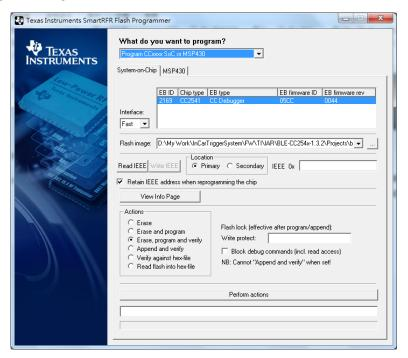
Correctly select the target device and make sure CC debugger is recognized by the flash programmer
