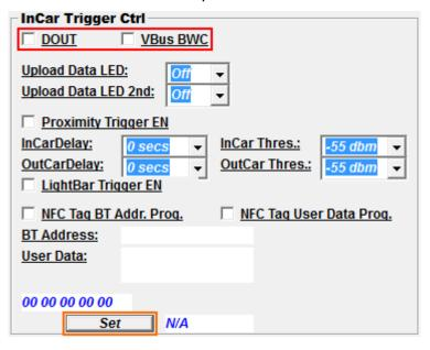
VBus\_2<sup>nd</sup> and CB\_2<sup>nd</sup> output is controlled based on the status of ignition input. These two output signal will be automatically pull high if state of ignition input is considered as logic high.
