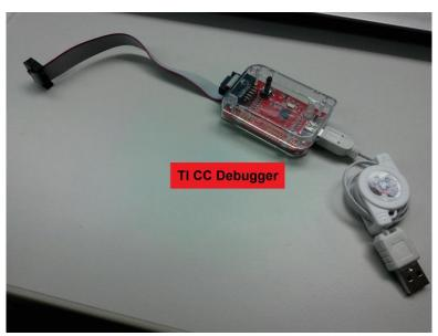
Texas Instruments **Smart RF Flash Programmer** software package contains the driver of CC debugger to let the connected host system to identify this device. Download and install the Smart RF Flash Programmer from Texas Instruments official Website http://www.ti.com/tool/flash-programmer.
