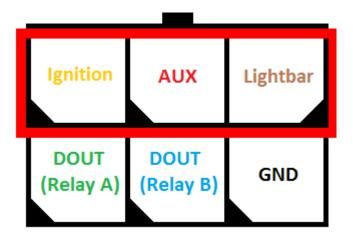
All these three digital input could sustain  $8V \sim 30V$  input voltage and controller of In-Car Trigger would determine the digital input as logic high level while apply voltage with this range.
