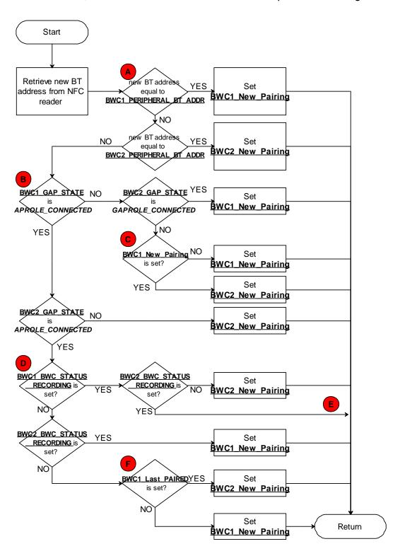
In the scenario (B), (C), (D), and (F) above, The buffered BWC mac address paired with allocated Bluetooth channel will be overwrite by the one of target BWC, and the original BWC should be re-paired to In-Car Trigger if it want to setup the Bluetooth connection to In-Car Trigger again.
