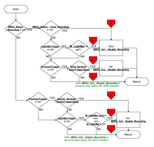
Base on the recording is turned on or off in received status of paired BWC, the remote recording control scenarios could be listed in the following cases tagged in the control flow above:
