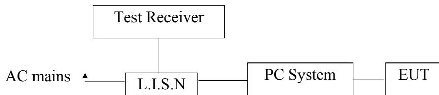
(EUT: Receiver of 2.4G Wireless Optical Mouse)
