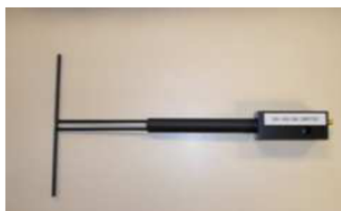
Figure 1 – Satimo COMOSAR Validation Dipole
