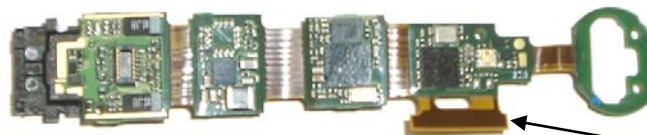
Bottom View of main PWB (Right Earpiece)
