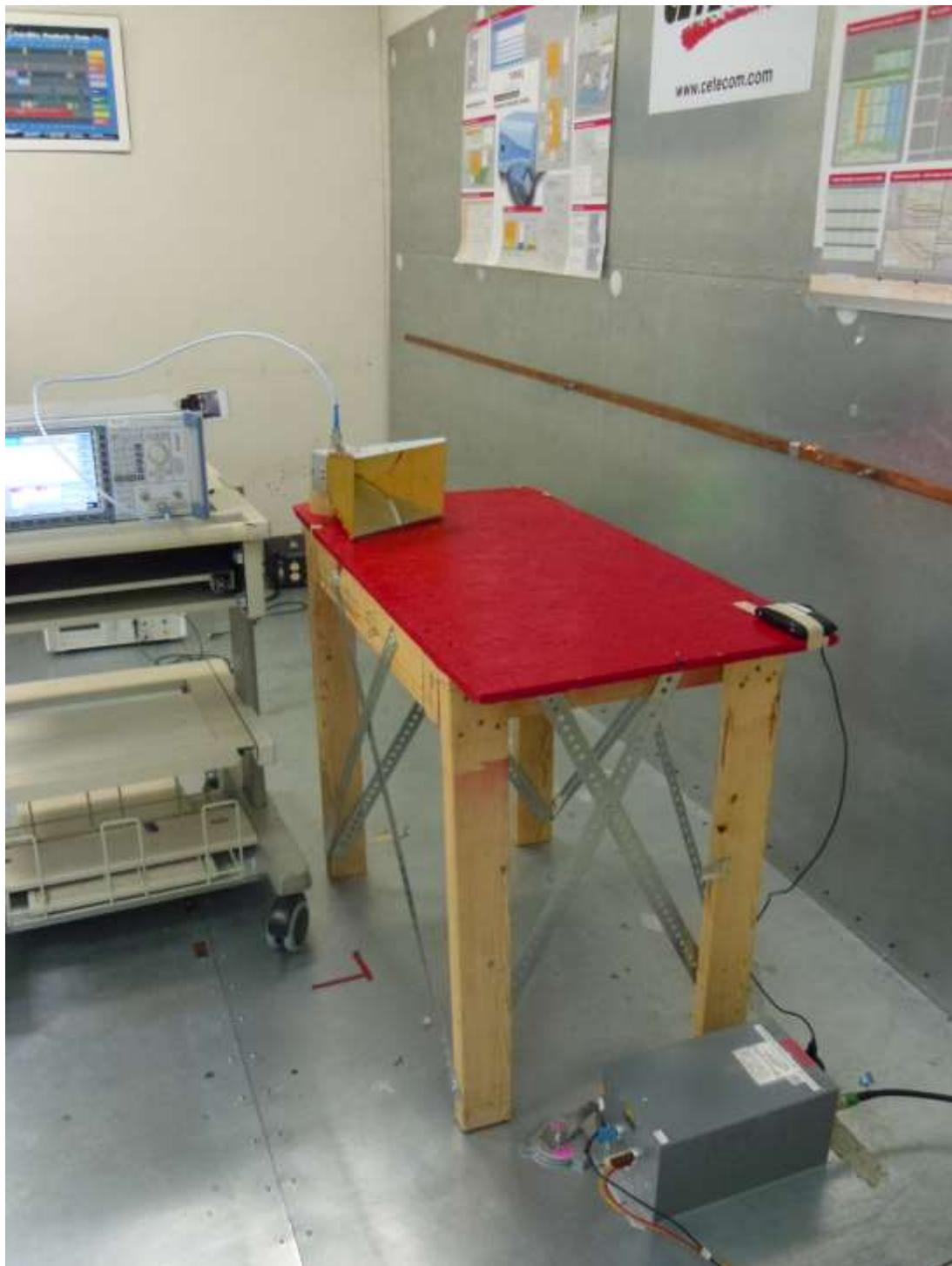
Radiated Test Setup:
