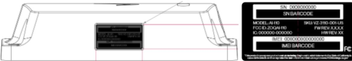
The label with S/N and IMEI barcodes is found on the side of the device, which allows it to be read even after mounting. You will scan the label when instructed in the Reveal Hardware Installer app, or if the scan should fail, enter the IMEI. The text on the device label is small, so if difficult to read, you can refer to the enlarged label found on the box that came with the device. The box label is also scannable.
