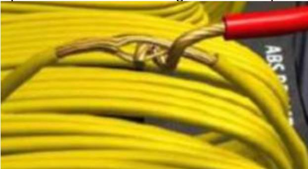
3. Press the wire back together then wrap the excess newly inserted wire tightly around it.
