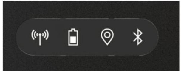
The device runs a status test for Battery, Network, and GPS whenever the status button is pressed. Status test results are displayed on the status LEDs as described below. The LEDs stay lit only for a brief duration. However, the test can be repeated by pressing the status button again, which is useful for determining the best place on the asset to mount the device.
