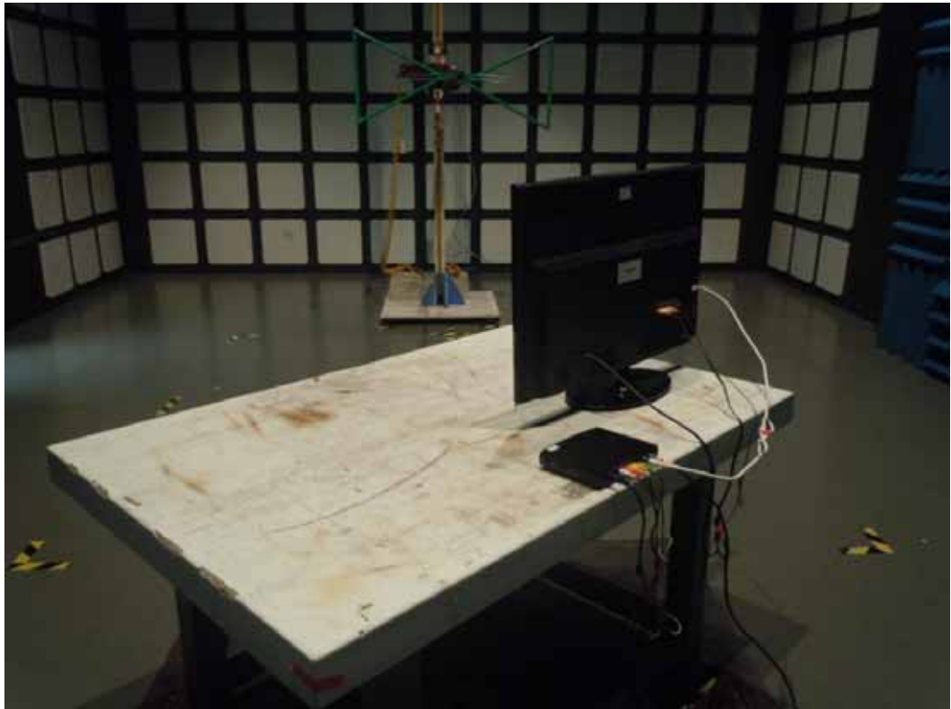
SETUP WITH MAXIMUM DETECTED EMISSION AT HORIZONTAL POLARIZATION (S/N: E1108987-01/02)
