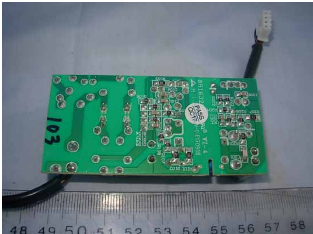
FIGURE 3 DIGITAL SET-TOP (M/N: CISCO 3413DVB) POWER BOARD #1 (SOLDERED SIDE)
