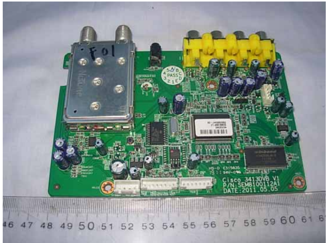
FIGURE 6 DIGITAL SET-TOP (M/N: CISCO 3413DVB) MAIN BOARD (COMPONENT SIDE)
