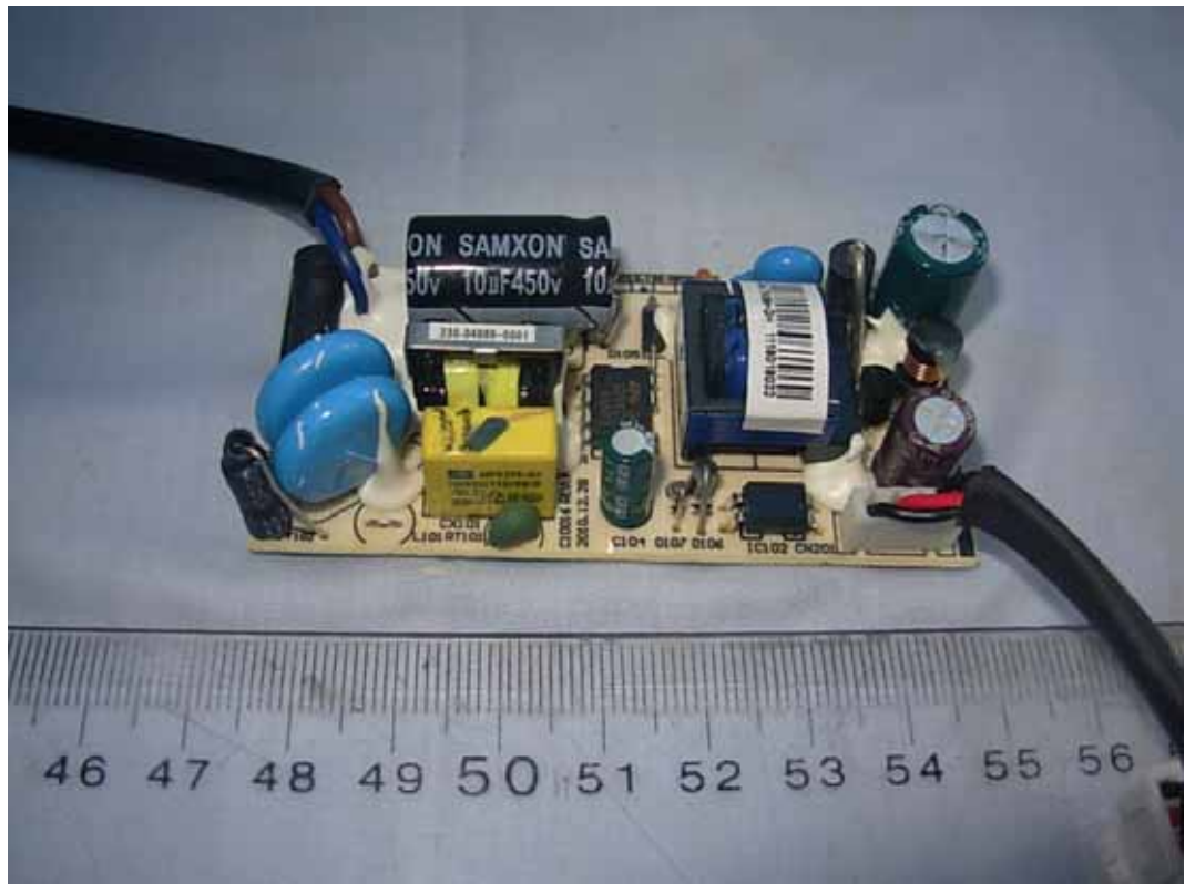
FIGURE 2 DIGITAL SET-TOP (M/N: CISCO 3413DVB) POWER BOARD #1 (COMPONENT SIDE)
