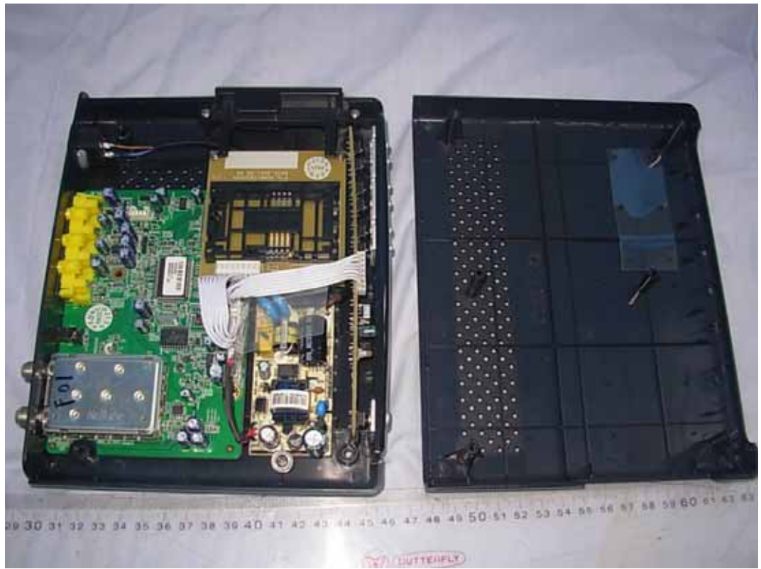
FIGURE 1 DIGITAL SET-TOP (M/N: CISCO 3413DVB) COVER REMOVED
