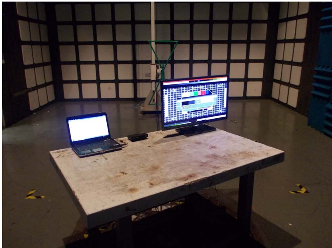
SETUP WITH MAXIMUM DETECTED EMISSION AT VERTICAL POLARIZATION (TEST MODE: AV MODE)
