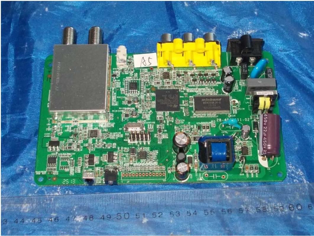
FIGURE 6 DIGITAL SET-TOP (M/N: PDS1100) MAIN BOARD (SOLDERED SIDE)
