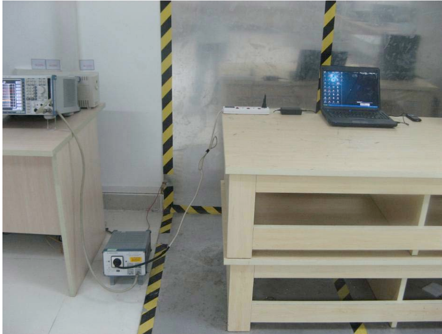
FCC LINE CONDUCTED EMISSION TEST SETUP
