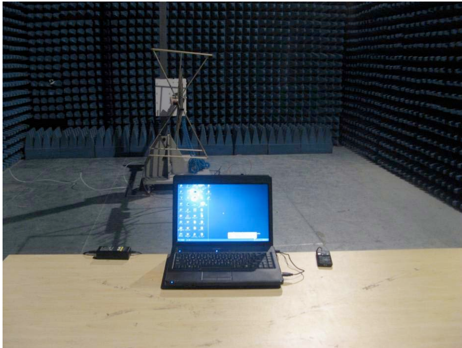
FCC RADIATED EMISSION TEST SETUP
