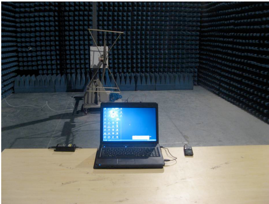
FCC RADIATED EMISSION TEST SETUP
