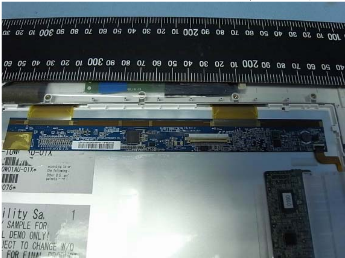
Figure 12 Internal View (Control Board, Front View)
