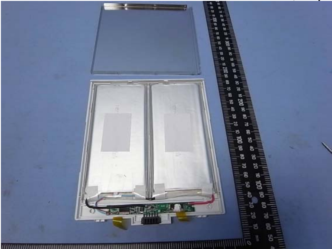
Figure 30 Internal View (Battery View)
