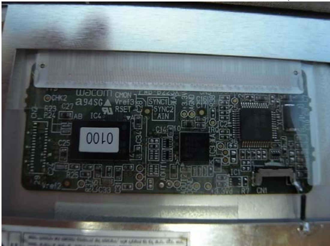
Figure 15 Internal View (Control Board)
