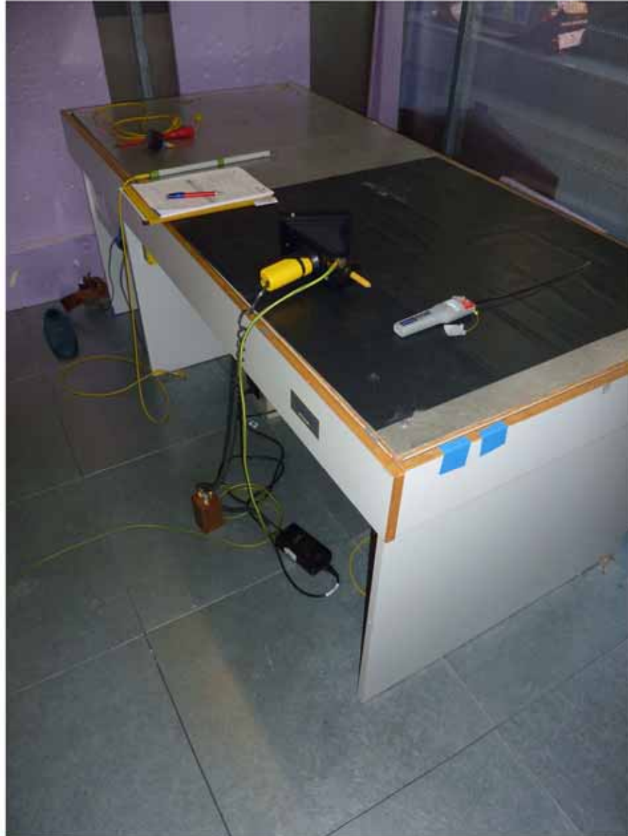
140898_1.jpg: Test setup ESD
