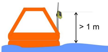
It is also possible to mount the easyRESCUE on the top of a pole with a fixture or the lanyard.
