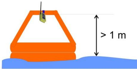
With the lanyard, which is included in the bracket, you can fix the easyRESCUE as high as possible at the life raft. Please ensure that the antenna height is more than 1 m above sea level.
