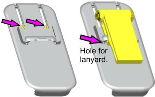
mounting plate starting from the wide side of the easyRESCUE and fix it with the screws. Then you can snap in the bracket. The both screws, the mounting plate and the bracket are included in the
