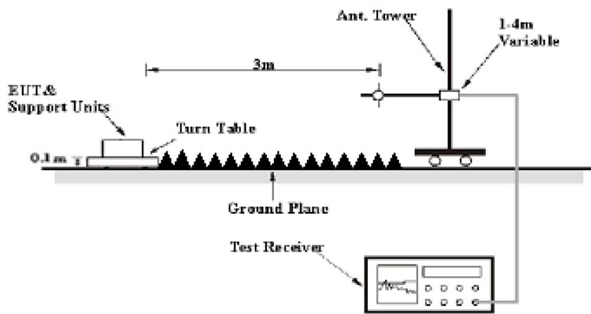
The radiated emission tests were performed in the 3 meters test site, using the setup accordance with the ANSI C63.4-2003. The specification used was the FCC 15.209, and FCC 15.247 limits.
