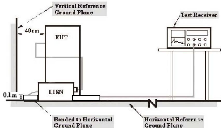
The setup of EUT is according with per ANSI C63.4-2003 measurement procedure. The specification used was with the FCC Part 15.207 limits.
