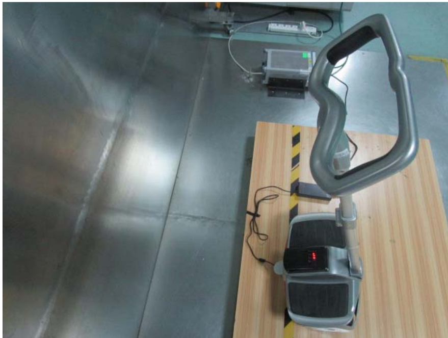
Conducted Emission - Side View
