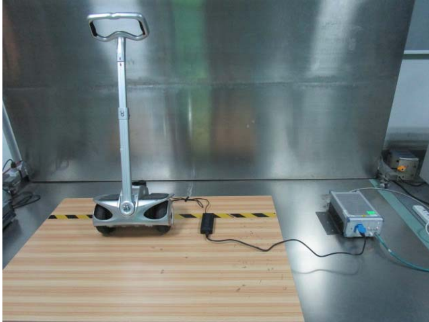
Conducted Emission - Side View
