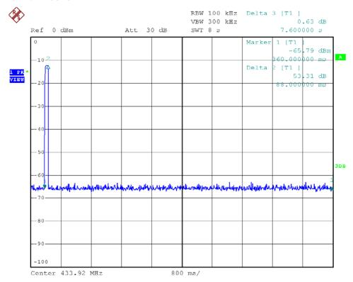
Note: "Marker 1" mean the moment button is pressed, and "Marker 2" mean where the button is released (no longer pressed). Then, from the plot, TX must be deactivated within 5 sec.
