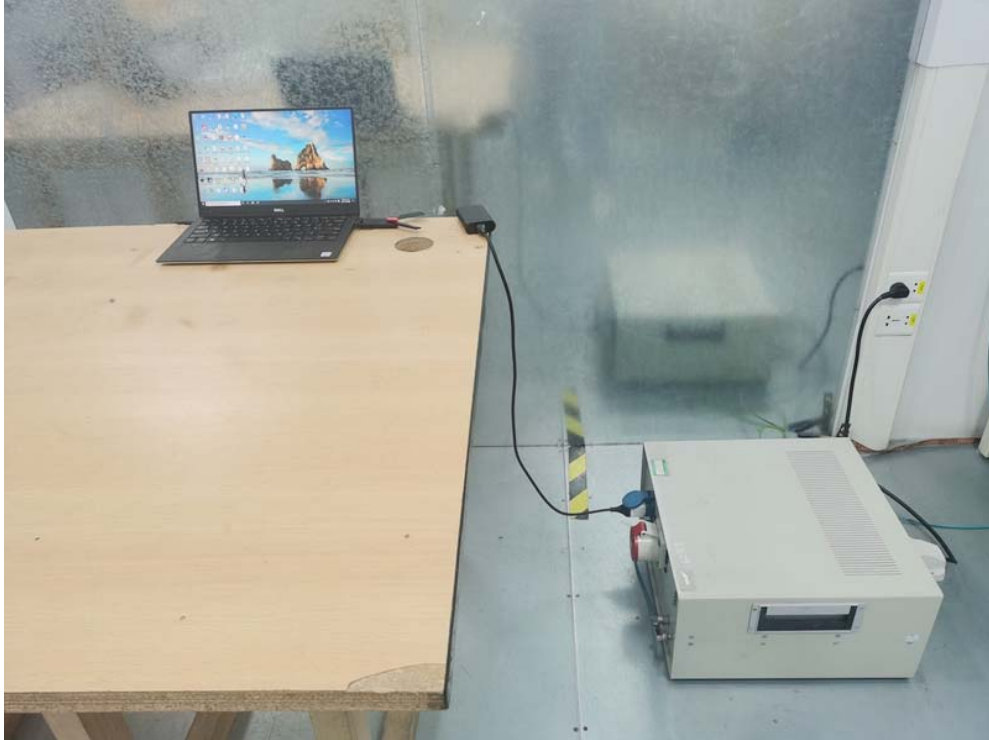
Conducted Emission Test Setup:
