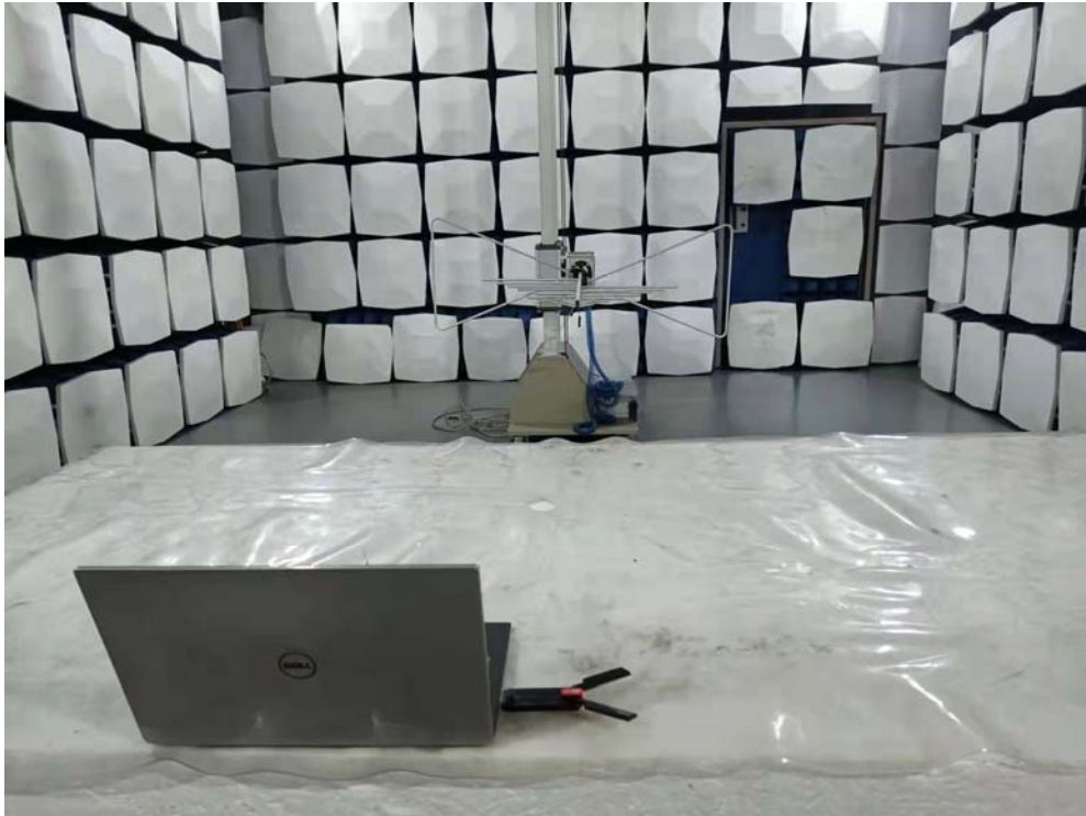
Radiated Emission Test Setup:
