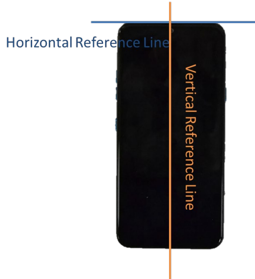
SAR Test Setup Photo 15 Vertical and Horizontal Reference Lines
