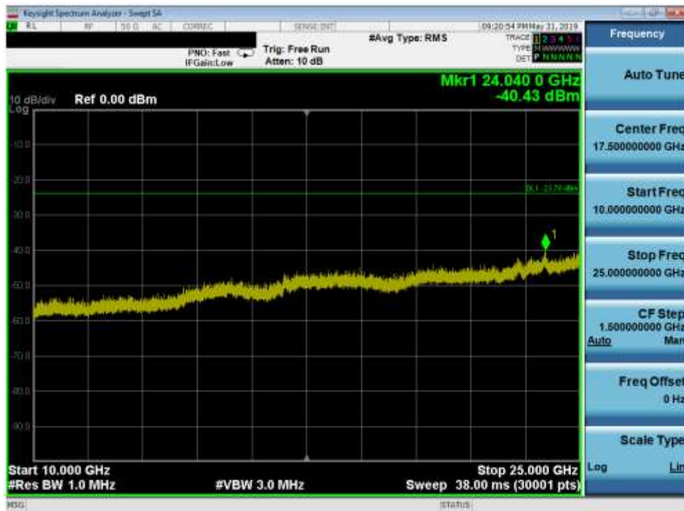
Plot 7-34. Conducted Spurious Plot (Bluetooth (LE), 2Mbps – Ch. 39)
