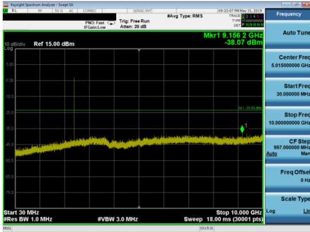
Plot 7-29. Conducted Spurious Plot (Bluetooth (LE), 2Mbps – Ch. 0)
