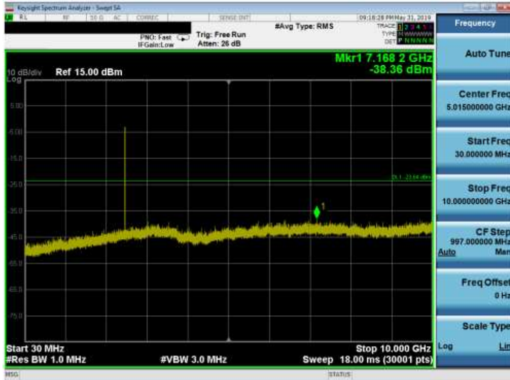
Plot 7-27. Conducted Spurious Plot (Bluetooth (LE), 1Mbps – Ch. 39)
