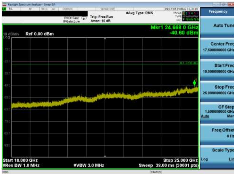
Plot 7-26. Conducted Spurious Plot (Bluetooth (LE), 1Mbps – Ch. 19)
