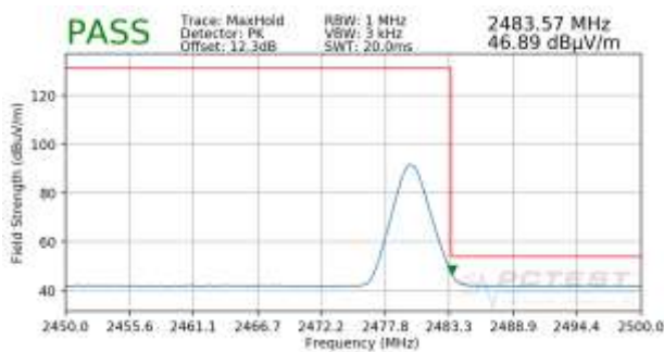
Plot 7-35. Radiated Restricted Upper Band Edge Measurement (Average)
