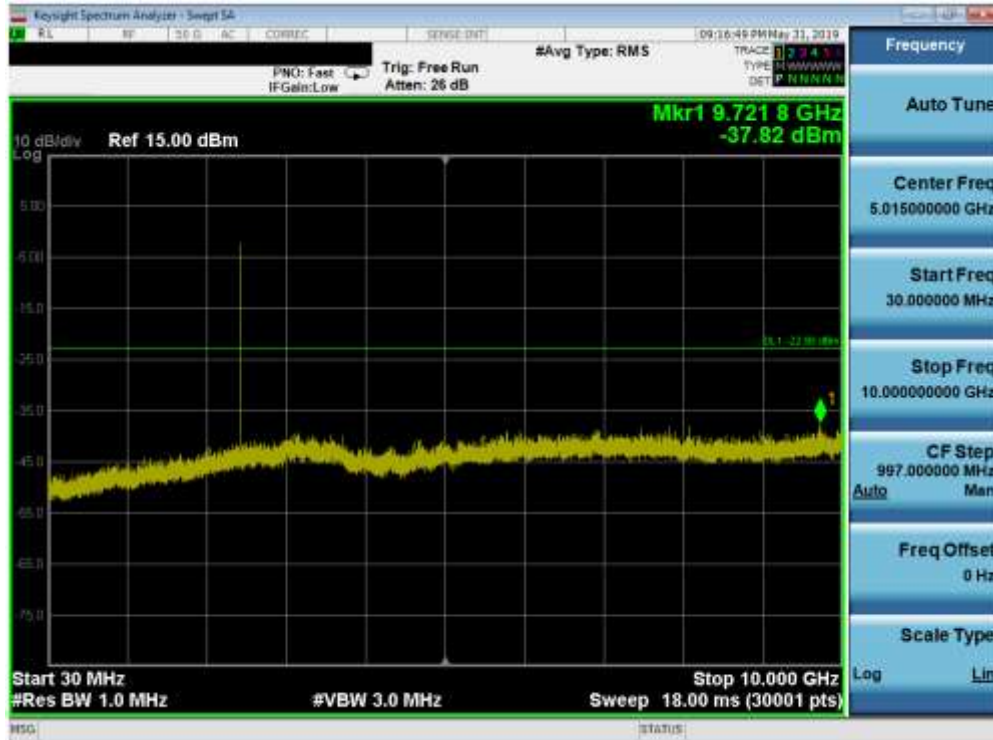
Plot 7-25. Conducted Spurious Plot (Bluetooth (LE), 1Mbps – Ch. 19)
