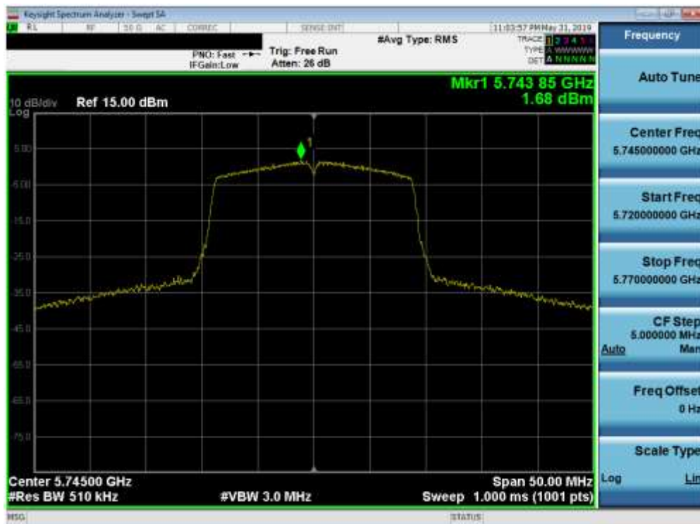
Plot 7-71. Power Spectral Density Plot (20MHz BW 802.11n (UNII Band 3) – Ch. 149)
