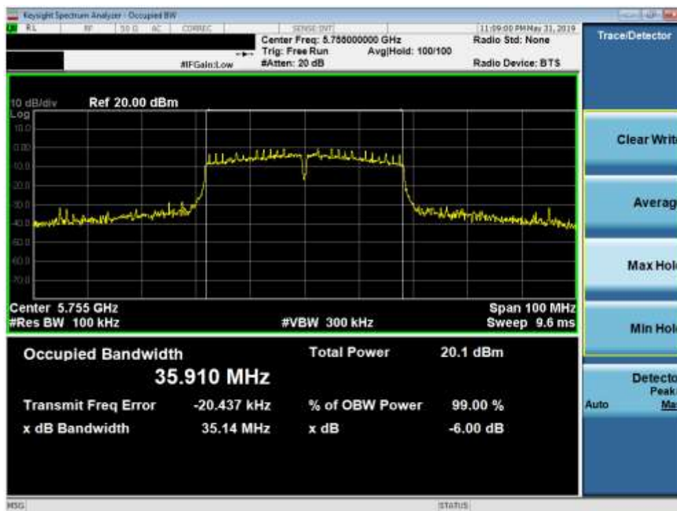
Plot 7-35. 6dB Bandwidth Plot (40MHz BW 802.11n (UNII Band 3) – Ch. 151)
