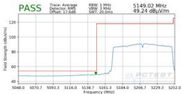
Plot 7-111. Radiated Lower Band Edge Plot (Average – UNII Band 1)
