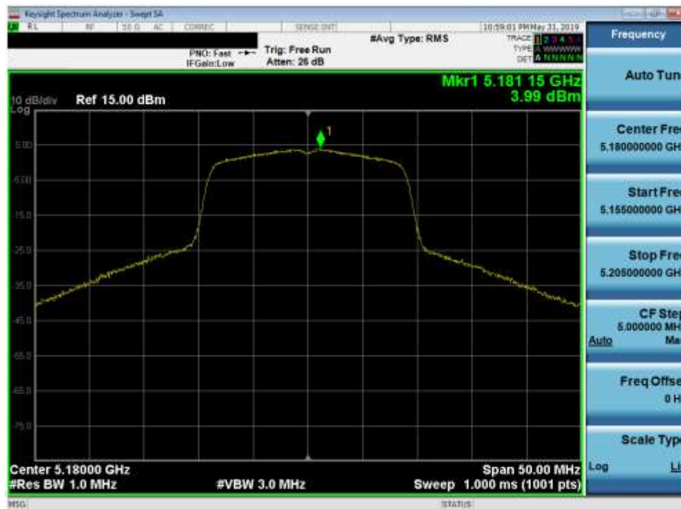
Plot 7-41. Power Spectral Density Plot (20MHz BW 802.11n (UNII Band 1) – Ch. 36)
