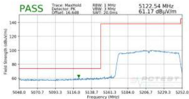
Plot 7-112. Radiated Lower Band Edge Plot (Peak – UNII Band 1)
