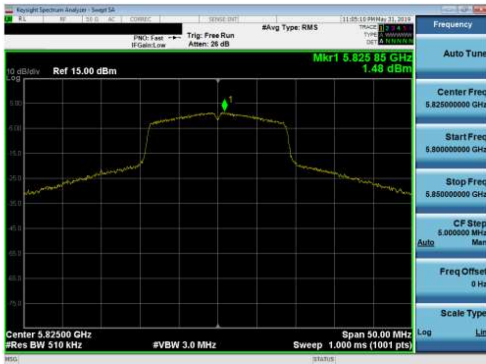
Plot 7-73. Power Spectral Density Plot (20MHz BW 802.11n (UNII Band 3) – Ch. 165)
