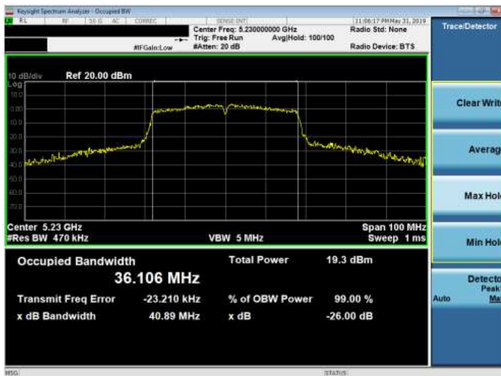
Plot 7-8. 26dB Bandwidth Plot (40MHz BW 802.11n (UNII Band 1) – Ch. 46)
