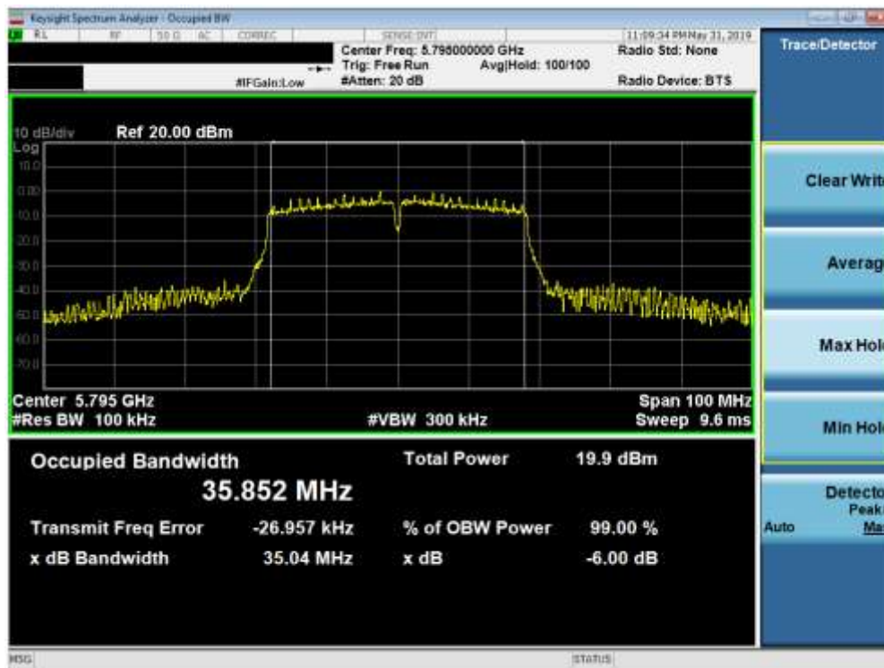
Plot 7-36. 6dB Bandwidth Plot (40MHz BW 802.11n (UNII Band 3) – Ch. 159)
