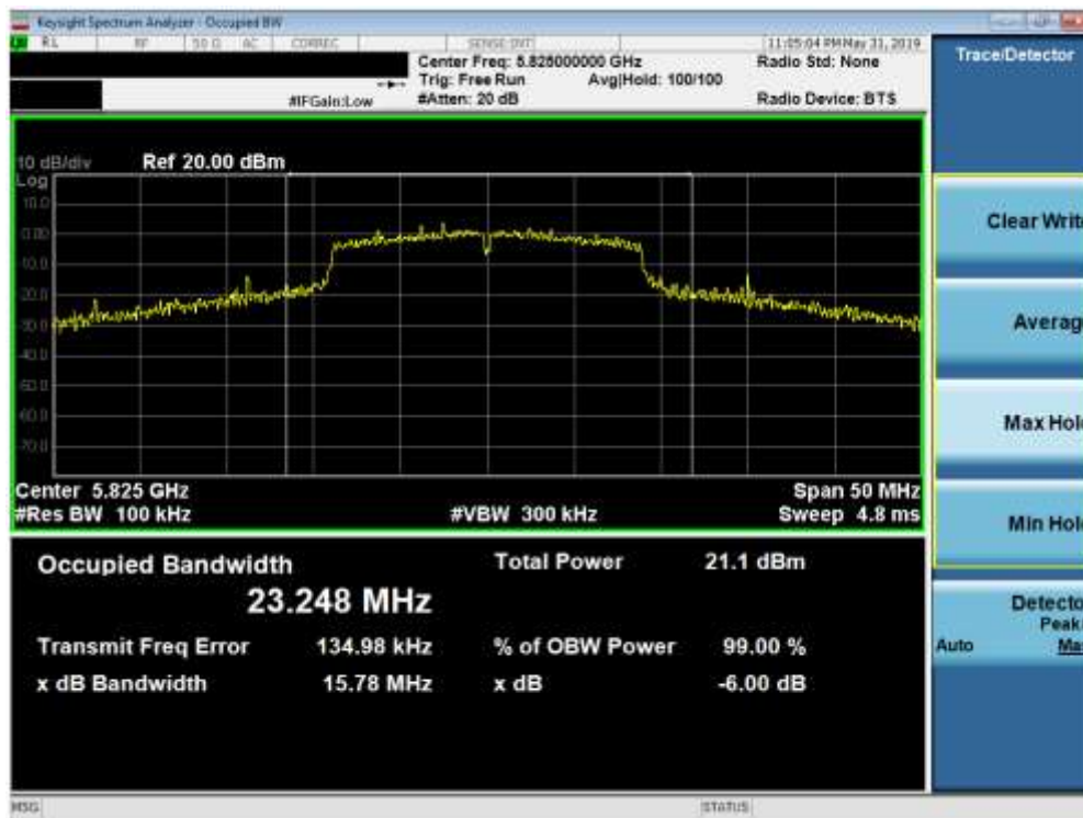
Plot 7-34. 6dB Bandwidth Plot (20MHz BW 802.11n (UNII Band 3) – Ch. 165)
