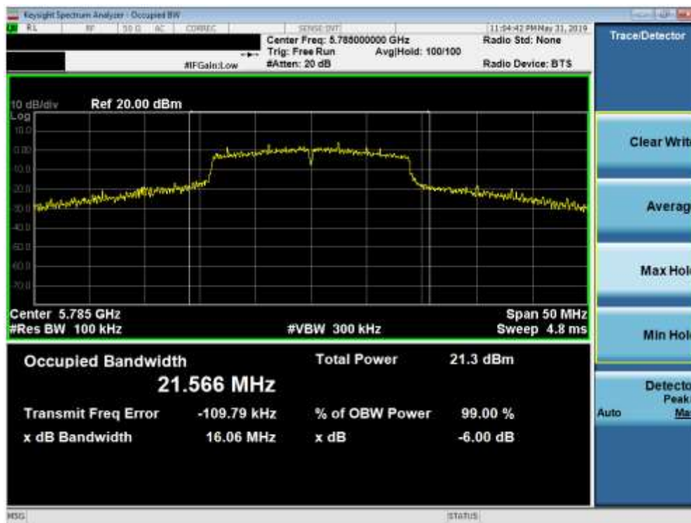
Plot 7-33. 6dB Bandwidth Plot (20MHz BW 802.11n (UNII Band 3) – Ch. 157)
