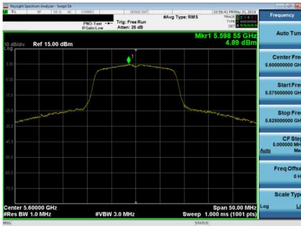
Plot 7-57. Power Spectral Density Plot (802.11a (UNII Band 2C) – Ch. 116)
