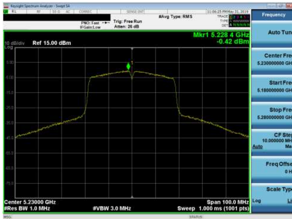
Plot 7-45. Power Spectral Density Plot (40MHz BW 802.11n (UNII Band 1) – Ch. 46)
