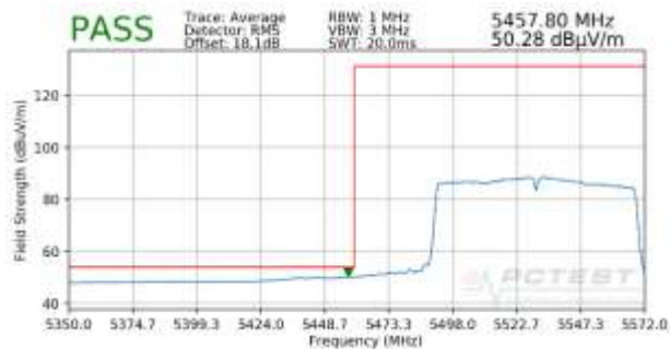
Plot 7-115. Radiated Lower Band Edge Plot (Average – UNII Band 2C)
