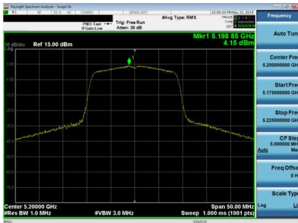
Plot 7-42. Power Spectral Density Plot (20MHz BW 802.11n (UNII Band 1) – Ch. 40)
