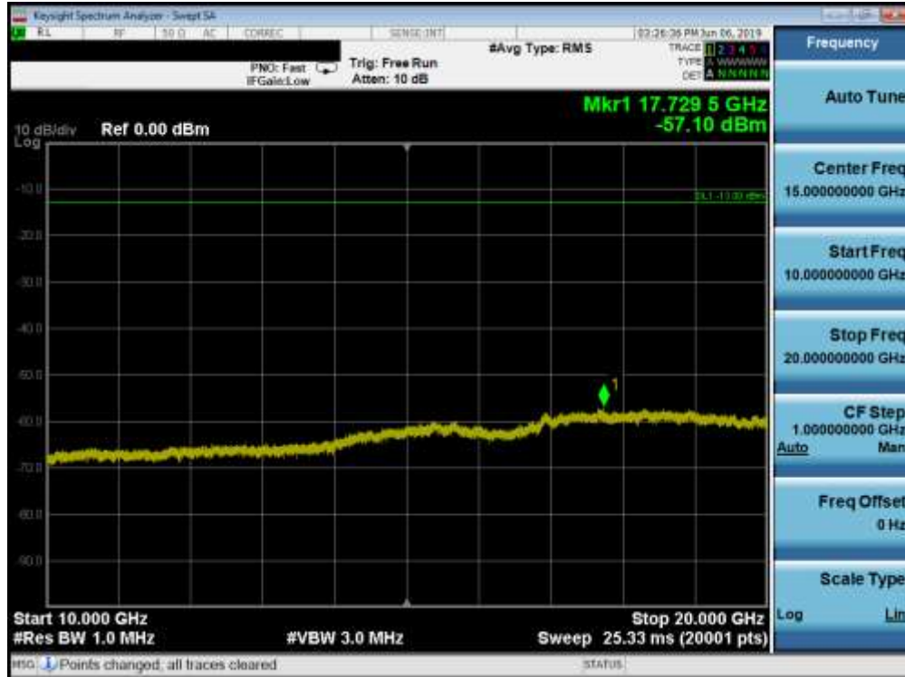
Plot 7-76. Conducted Spurious Plot (Band 66/4 - 20.0MHz QPSK - RB Size 1, RB Offset 0 - Low Channel)
