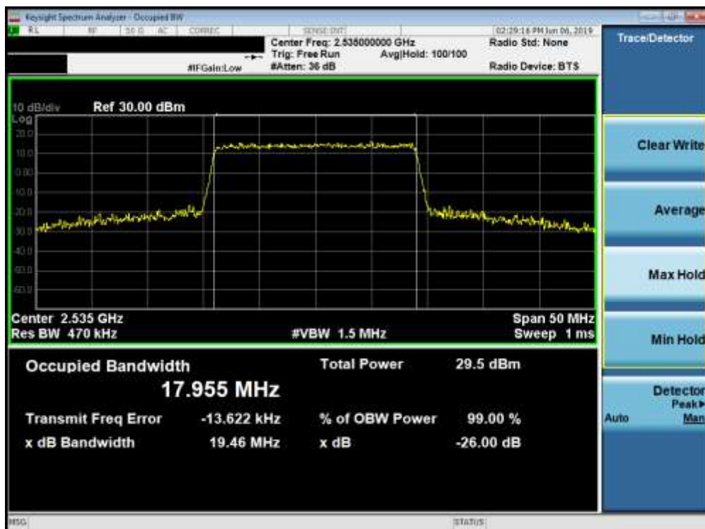
Plot 7-52. Occupied Bandwidth Plot (Band 7 - 20.0MHz 16-QAM - Full RB Configuration)
