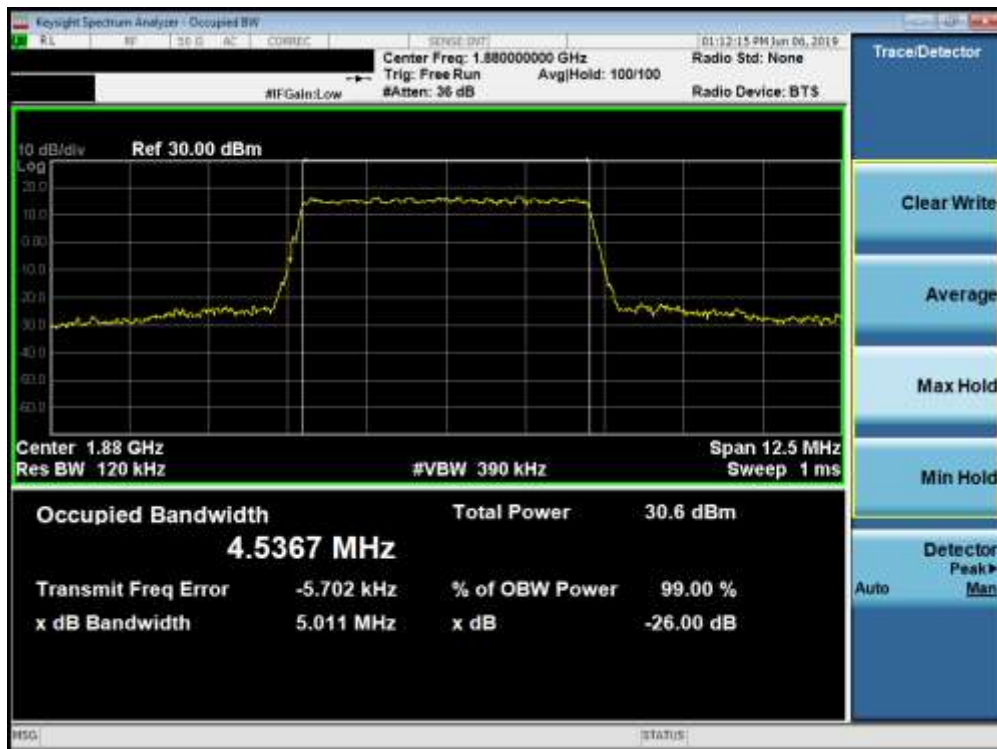
Plot 7-37. Occupied Bandwidth Plot (Band 2 - 5.0MHz QPSK - Full RB Configuration)
