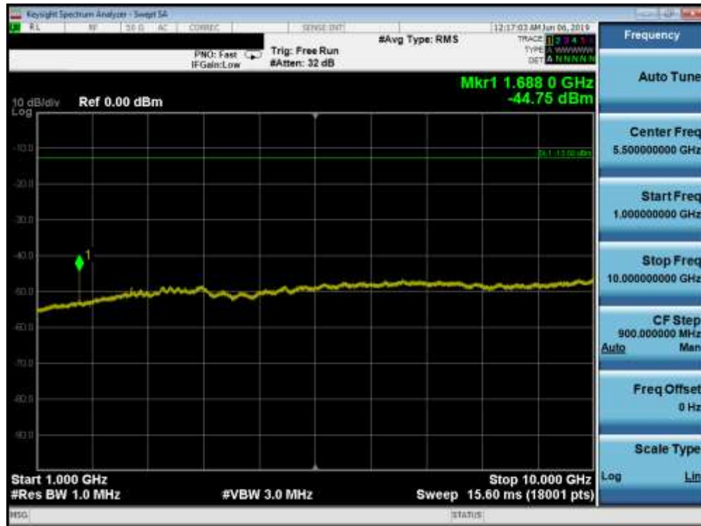
Plot 7-73. Conducted Spurious Plot (Band 5 - 10.0MHz QPSK - RB Size 1, RB Offset 0 - High Channel)
