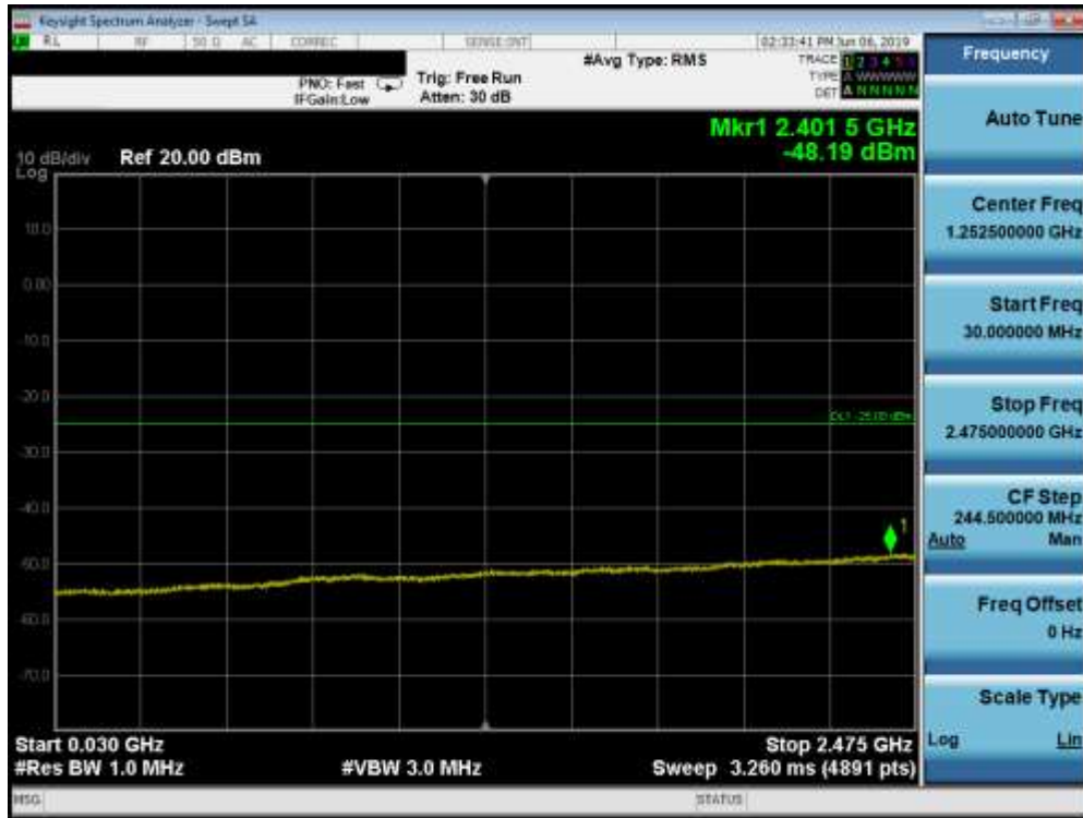
Plot 7-92. Conducted Spurious Plot (Band 7 - 20.0MHz QPSK - RB Size 1, RB Offset 0 - Low Channel)
