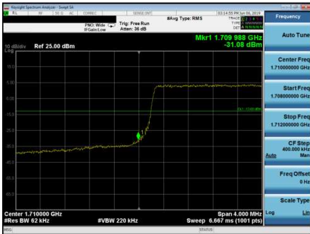
Plot 7-139. Lower Band Edge Plot (Band 66/4 - 5.0MHz QPSK - Full RB Configuration)
