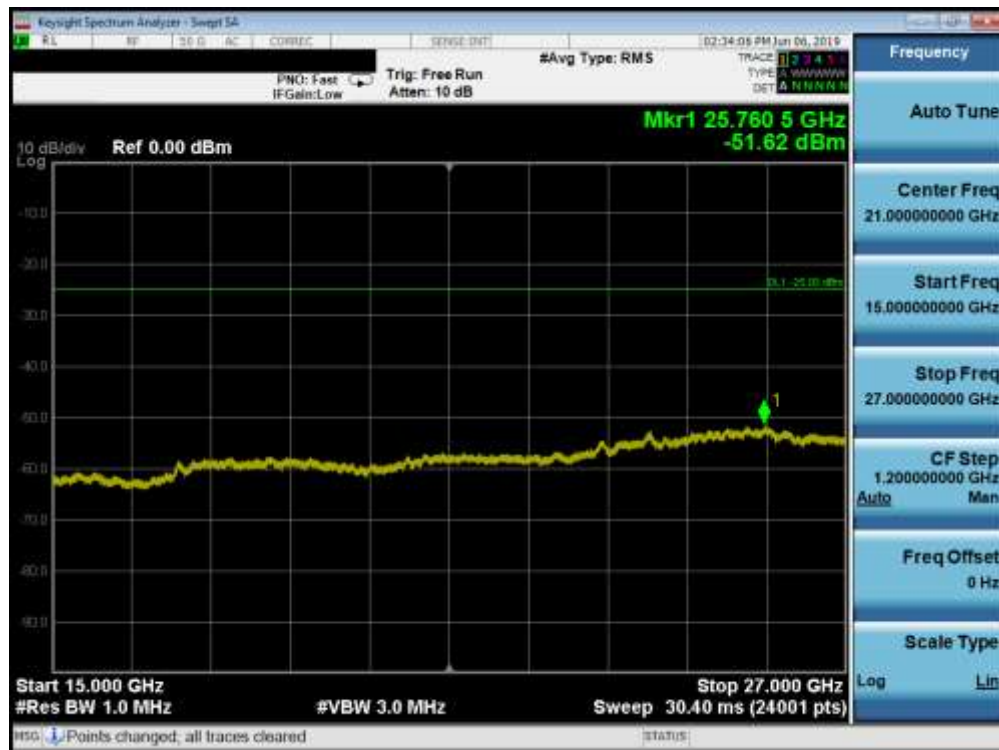
Plot 7-94. Conducted Spurious Plot (Band 7 - 20.0MHz QPSK - RB Size 1, RB Offset 0 - Low Channel)
