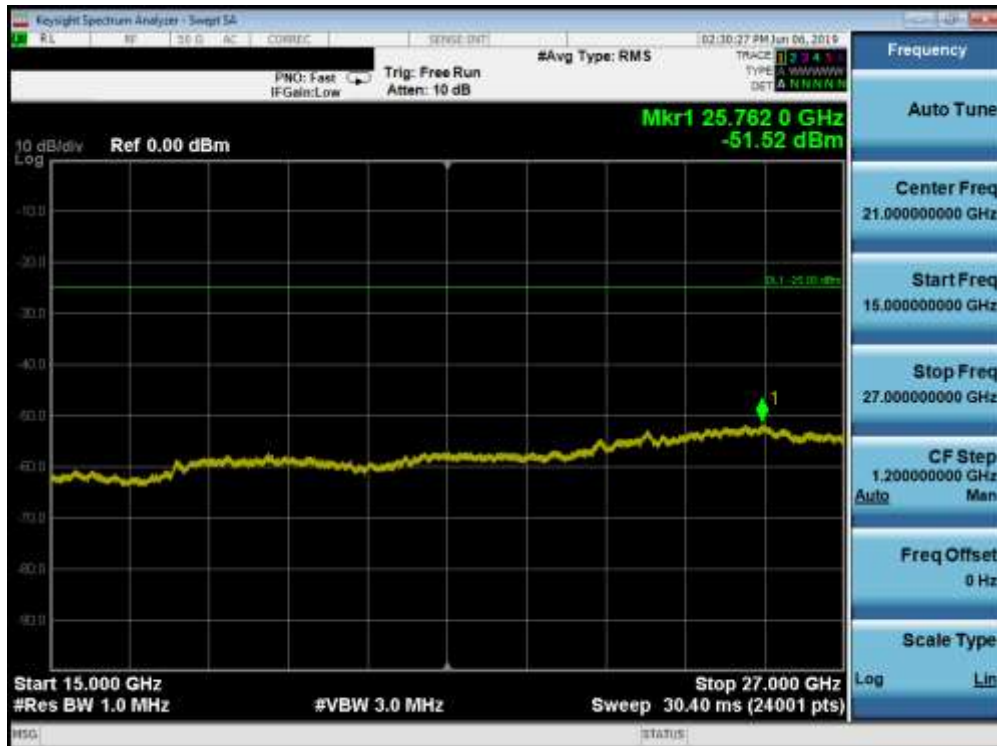
Plot 7-97. Conducted Spurious Plot (Band 7 - 20.0MHz QPSK - RB Size 1, RB Offset 0 - Mid Channel)
