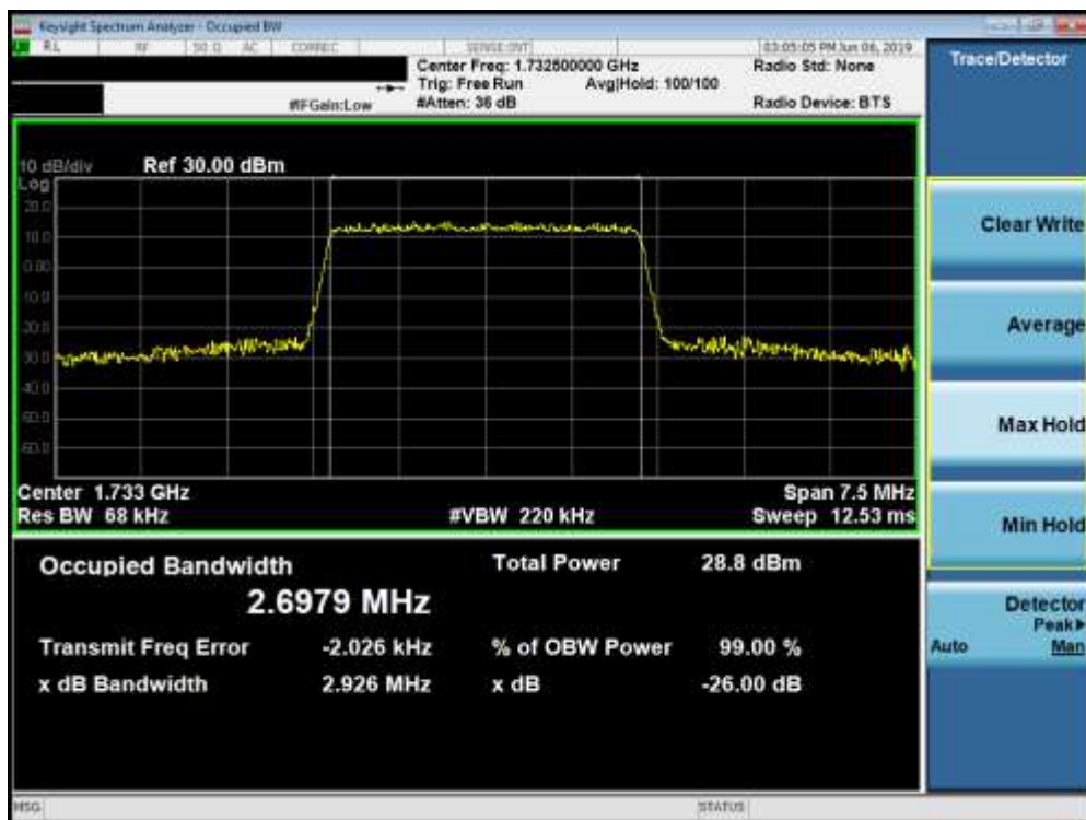
Plot 7-24. Occupied Bandwidth Plot (Band 66/4 - 3.0MHz 16-QAM - Full RB Configuration)
