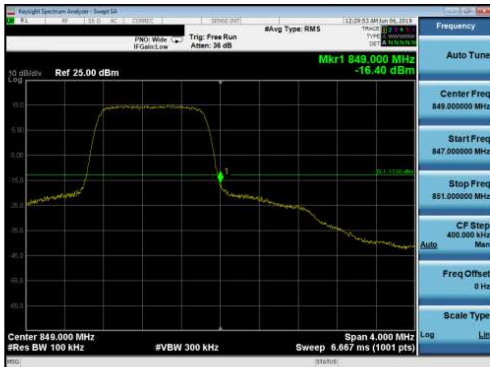
Plot 7-120. Upper Band Edge Plot (Band 5 - 1.4MHz QPSK - Full RB Configuration)
