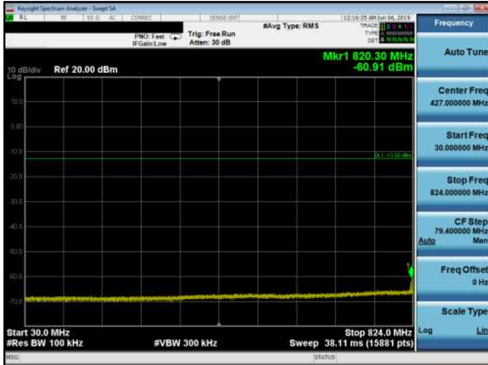
Plot 7-71. Conducted Spurious Plot (Band 5 - 10.0MHz QPSK - RB Size 1, RB Offset 0 - High Channel)
