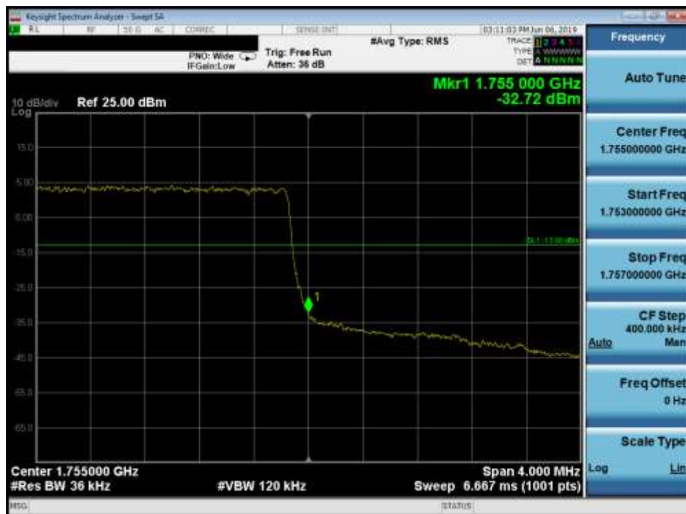
Plot 7-135. Upper Band Edge Plot (Band 4 - 3.0MHz QPSK - Full RB Configuration)
