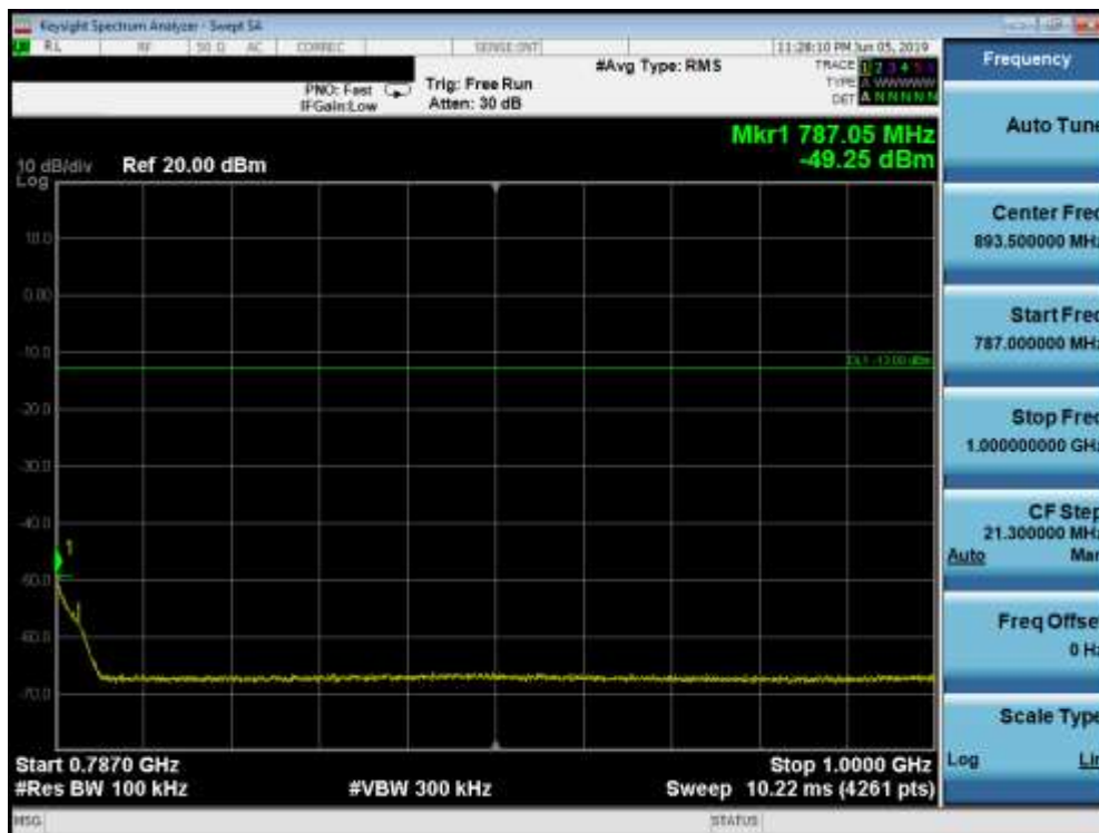
Plot 7-63. Conducted Spurious Plot (Band 13 - 10.0MHz QPSK - RB Size 1, RB Offset 0)
