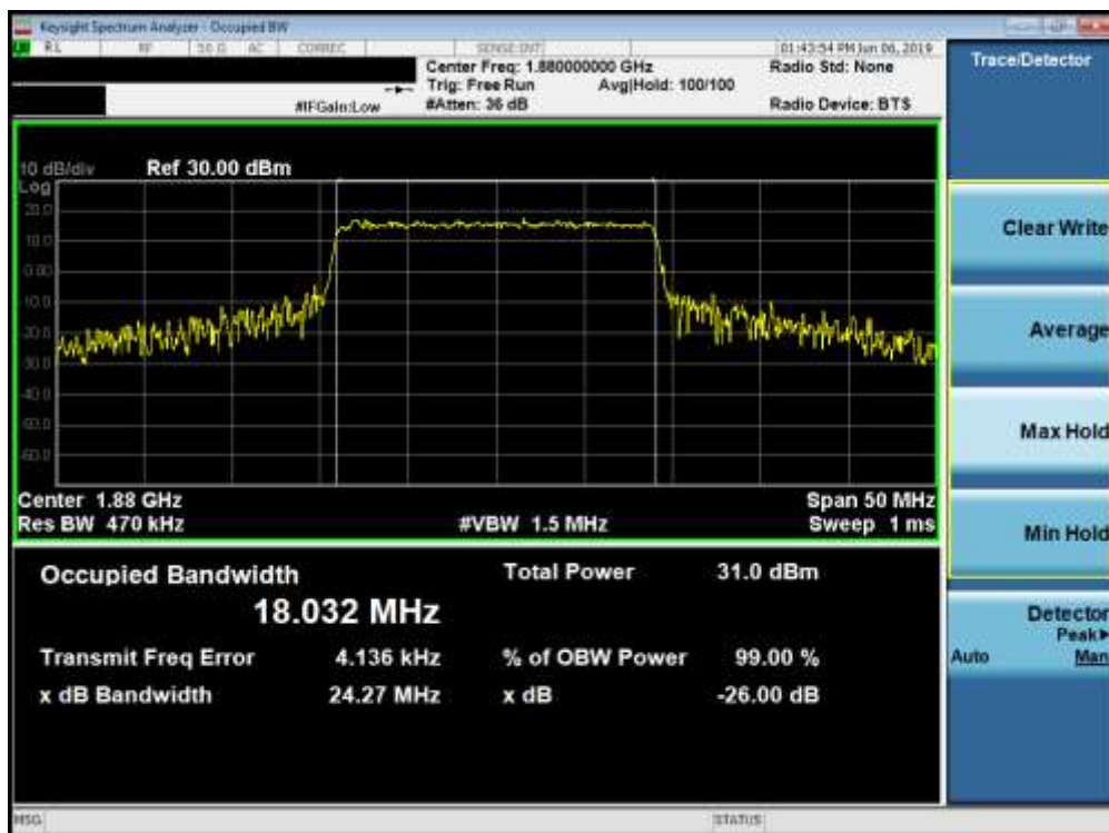
Plot 7-43. Occupied Bandwidth Plot (Band 2 - 20.0MHz QPSK - Full RB Configuration)
