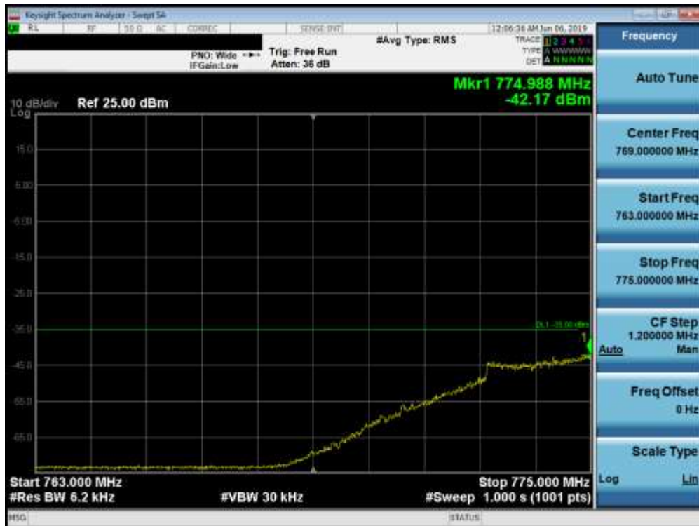
Plot 7-112. Lower Emission Mask Plot (Band 13 - 5.0MHz QPSK - Full RB Configuration)
