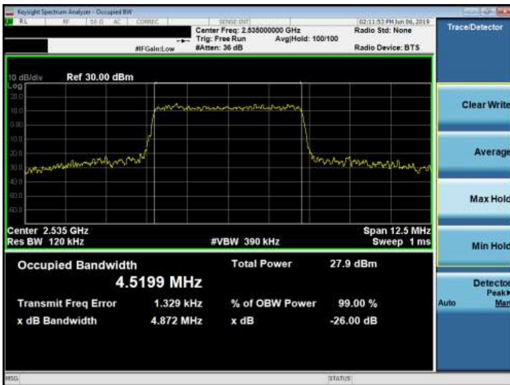
Plot 7-46. Occupied Bandwidth Plot (Band 7 - 5.0MHz 16-QAM - Full RB Configuration)
