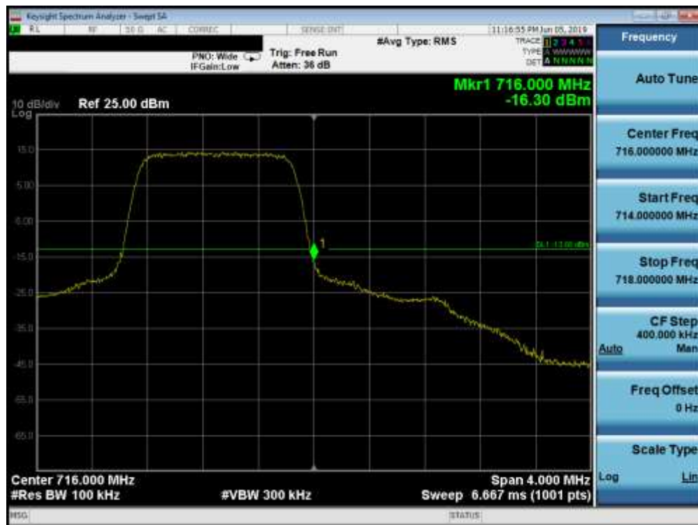
Plot 7-102. Upper Band Edge Plot (Band 12 - 1.4MHz QPSK - Full RB Configuration)
