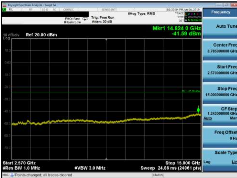
Plot 7-93. Conducted Spurious Plot (Band 7 - 20.0MHz QPSK - RB Size 1, RB Offset 0 - Low Channel)
