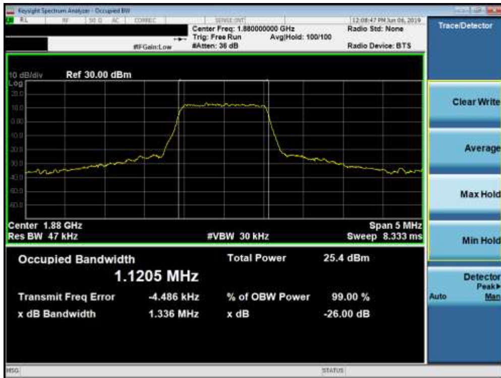
Plot 7-33. Occupied Bandwidth Plot (Band 2 - 1.4MHz QPSK - Full RB Configuration)
