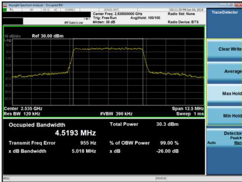
Plot 7-45. Occupied Bandwidth Plot (Band 7 - 5.0MHz QPSK - Full RB Configuration)
