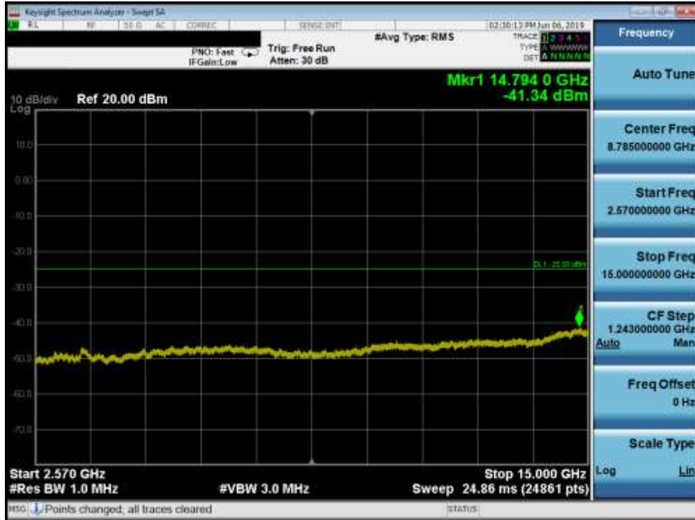
Plot 7-96. Conducted Spurious Plot (Band 7 - 20.0MHz QPSK - RB Size 1, RB Offset 0 - Mid Channel)
