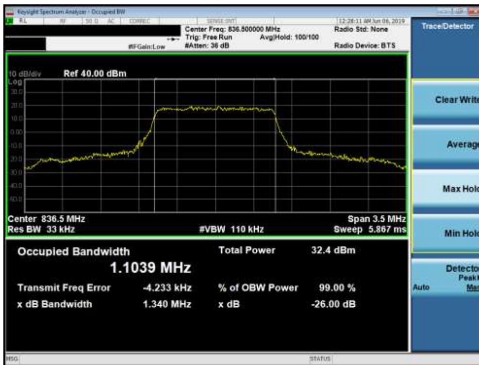
Plot 7-13. Occupied Bandwidth Plot (Band 5 - 1.4MHz QPSK - Full RB Configuration)
