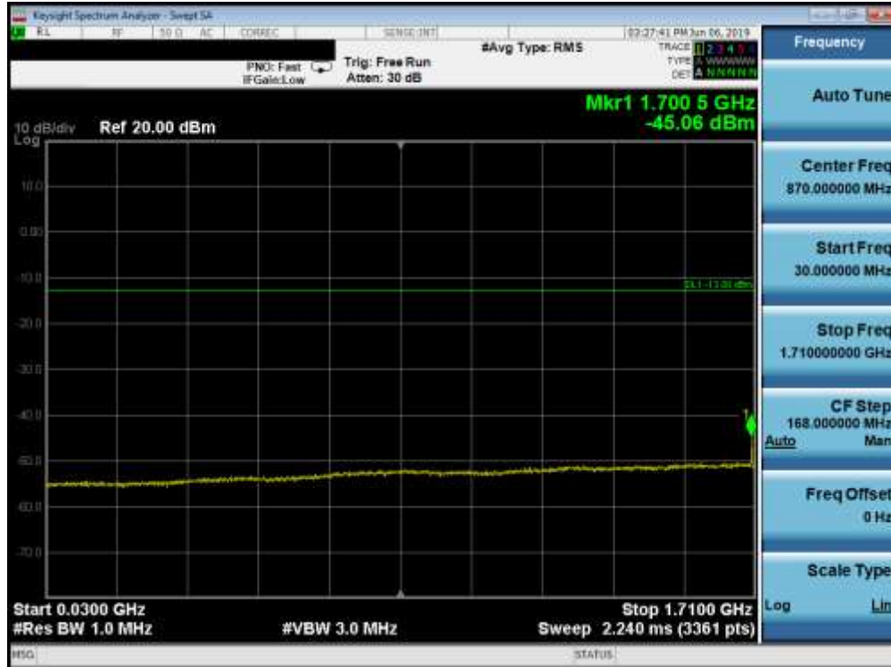
Plot 7-80. Conducted Spurious Plot (Band 66/4 - 20.0MHz QPSK - RB Size 1, RB Offset 0 - High Channel)
