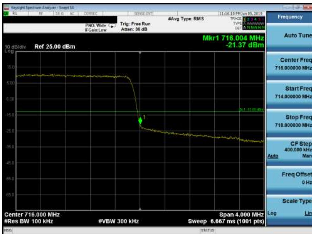
Plot 7-104. Upper Band Edge Plot (Band 12 - 3.0MHz QPSK - Full RB Configuration)
