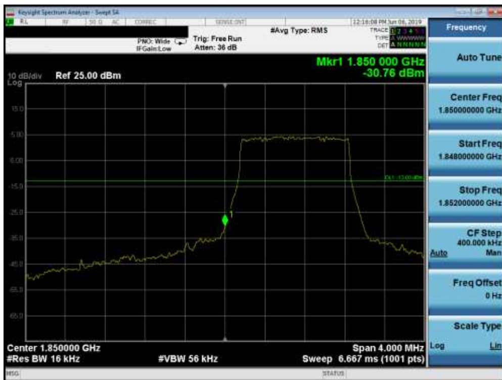
Plot 7-163. Lower Band Edge Plot (Band 2 - 1.4MHz QPSK - Full RB Configuration)
