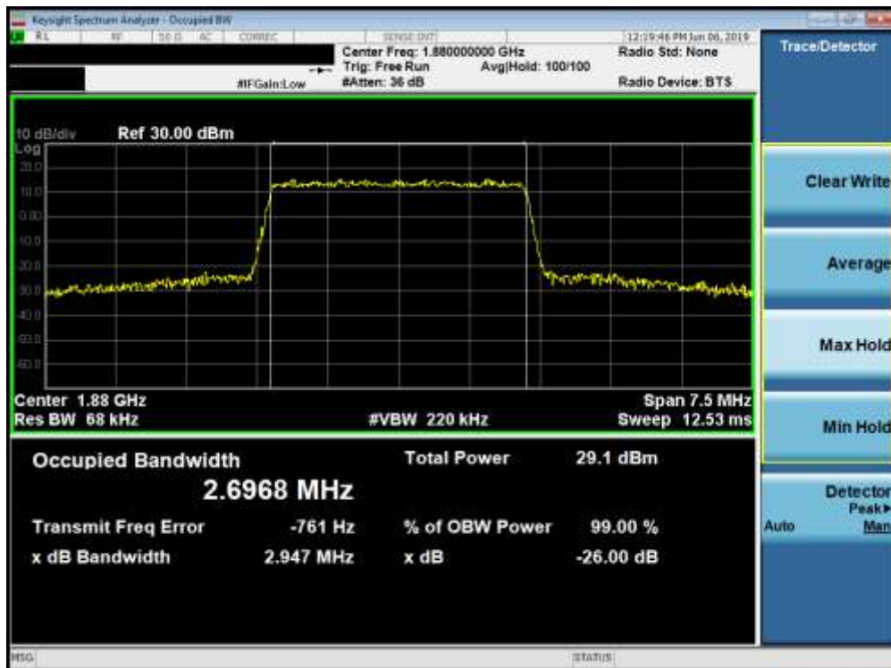
Plot 7-36. Occupied Bandwidth Plot (Band 2 - 3.0MHz 16-QAM - Full RB Configuration)
