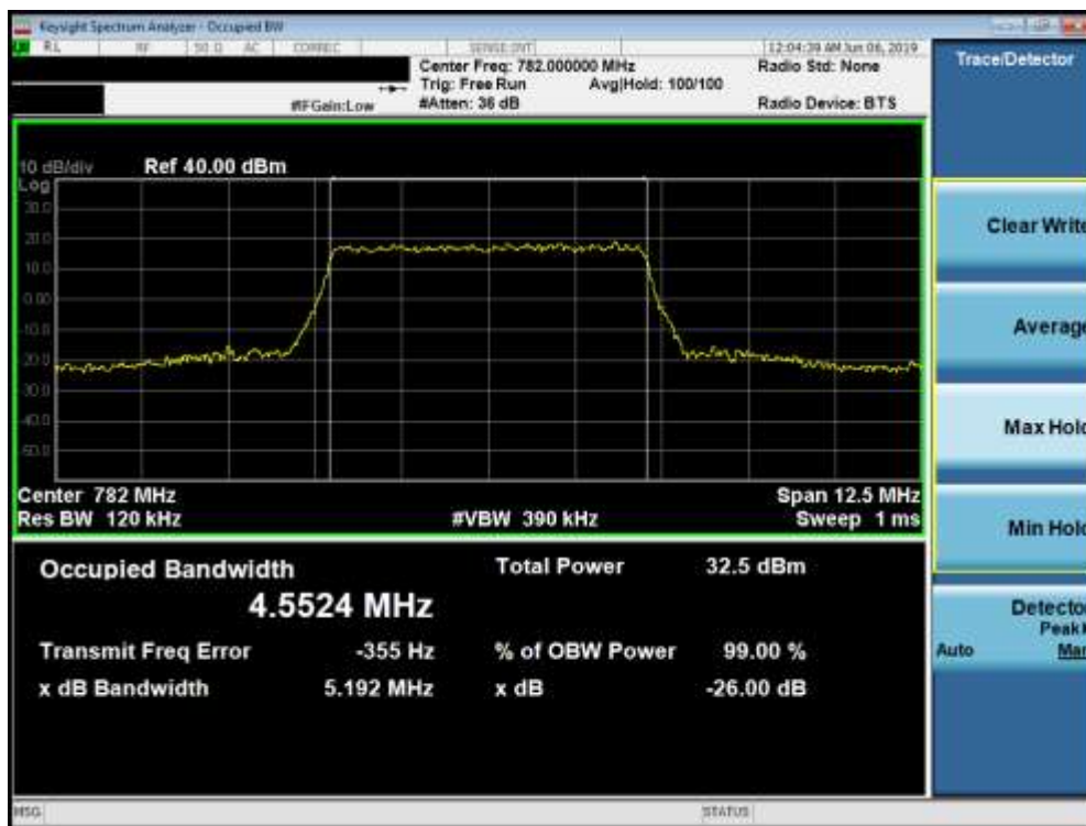
Plot 7-9. Occupied Bandwidth Plot (Band 13 - 5.0MHz QPSK - Full RB Configuration)
