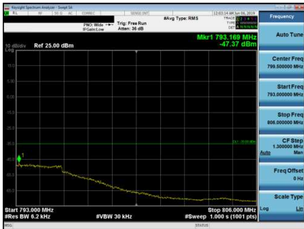
Plot 7-118. Upper Emission Mask Plot (Band 13 - 10.0MHz QPSK - Full RB Configuration)
