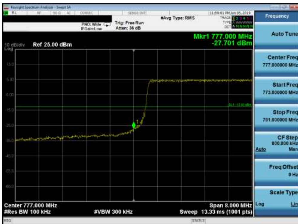
Plot 7-115. Lower Band Edge Plot (Band 13 - 10.0MHz QPSK - Full RB Configuration)
