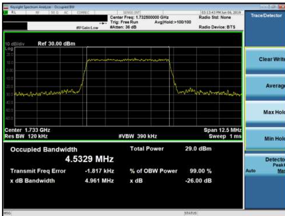
Plot 7-26. Occupied Bandwidth Plot (Band 66/4 - 5.0MHz 16-QAM - Full RB Configuration)
