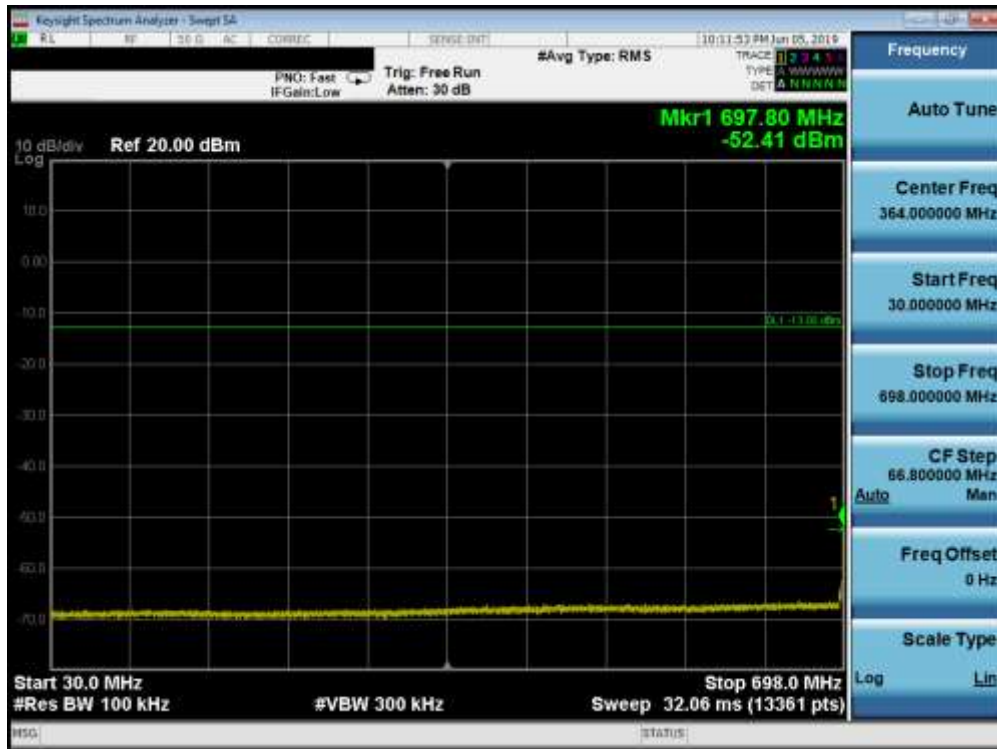
Plot 7-59. Conducted Spurious Plot (Band 12/17 - 10.0MHz QPSK - RB Size 1, RB Offset 0 - High Channel)
