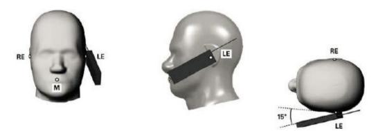
Fig.8.4 Illustration for Tilted Position
