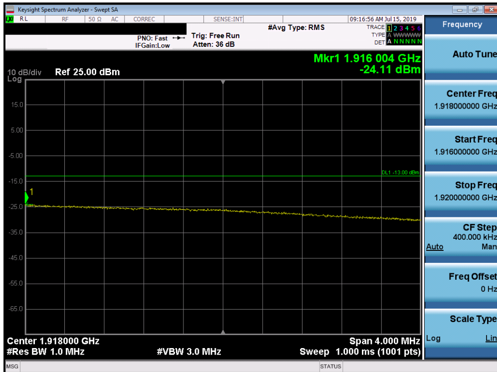
Plot 7-263. Upper Extended Band Edge Plot (Band 25 - 15.0MHz QPSK - Full RB Configuration)
