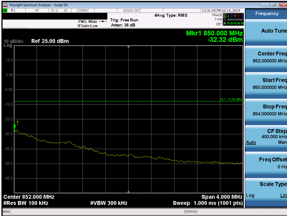
Plot 7-188. Upper Extended Band Edge Plot (Band 26/5 - 1.4MHz QPSK - Full RB Configuration)
