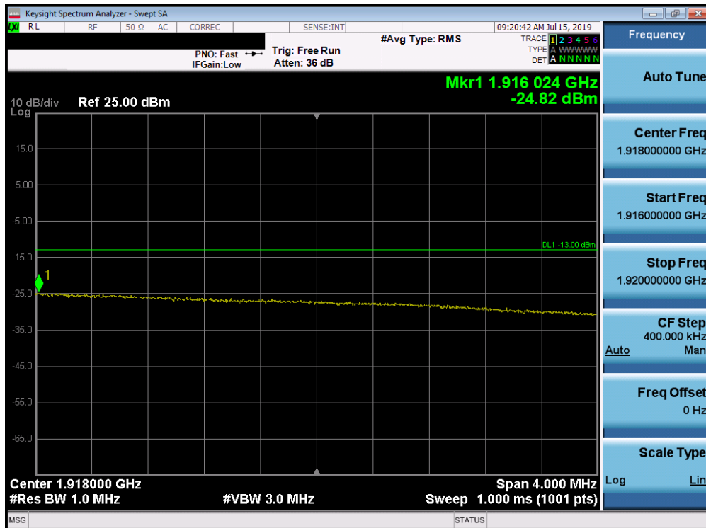
Plot 7-269. Upper Extended Band Edge Plot (Band 25 - 20.0MHz QPSK - Full RB Configuration)
