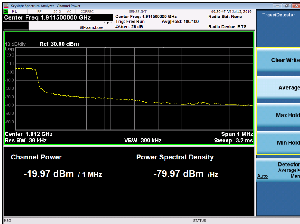
Plot 7-243. Upper Extended Band Edge Plot (Band 2 - 3.0MHz QPSK - Full RB Configuration)
