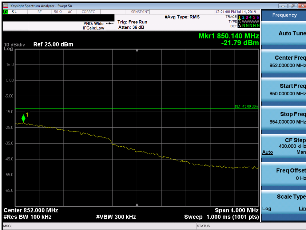
Plot 7-191. Upper Extended Band Edge Plot (Band 26/5 - 3.0MHz QPSK - Full RB Configuration)
