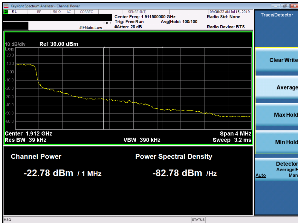
Plot 7-237. Upper Extended Band Edge Plot (Band 2 - 1.4MHz QPSK - Full RB Configuration)
