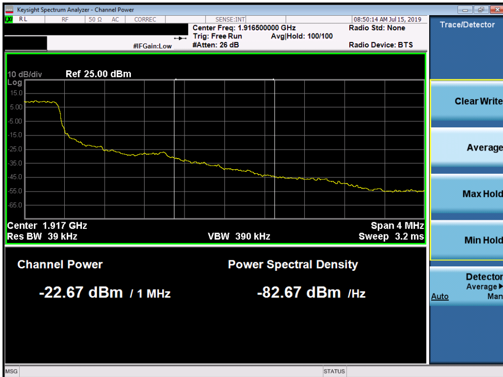
Plot 7-239. Upper Extended Band Edge Plot (Band 25 - 1.4MHz QPSK - Full RB Configuration)
