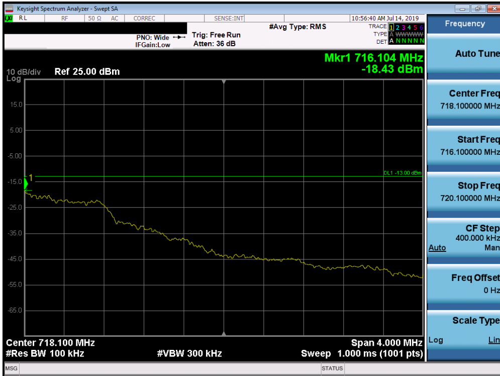
Plot 7-173. Upper Extended Band Edge Plot (Band 12 - 1.4MHz QPSK - Full RB Configuration)
