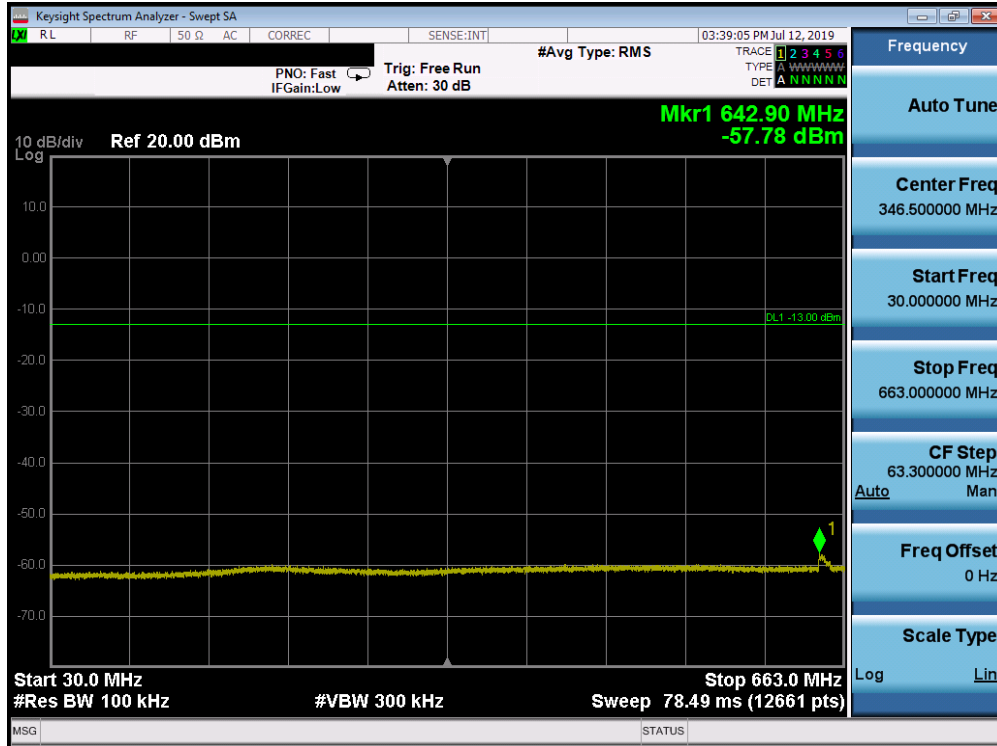
Plot 7-112. Conducted Spurious Plot (Band 71 - 10.0MHz QPSK - RB Size 1, RB Offset 0 - High Channel)
