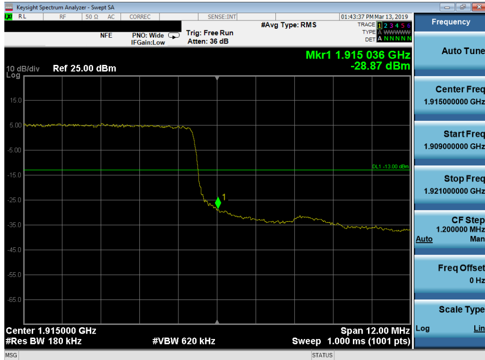
Plot 7-182. Upper Band Edge Plot (Band 25 - 15.0MHz QPSK - Full RB Configuration)
