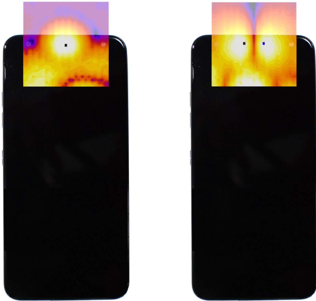
Figure 15-4 OTT VoIP T-Coil Scan Overlay Magnetic Field Distributions
