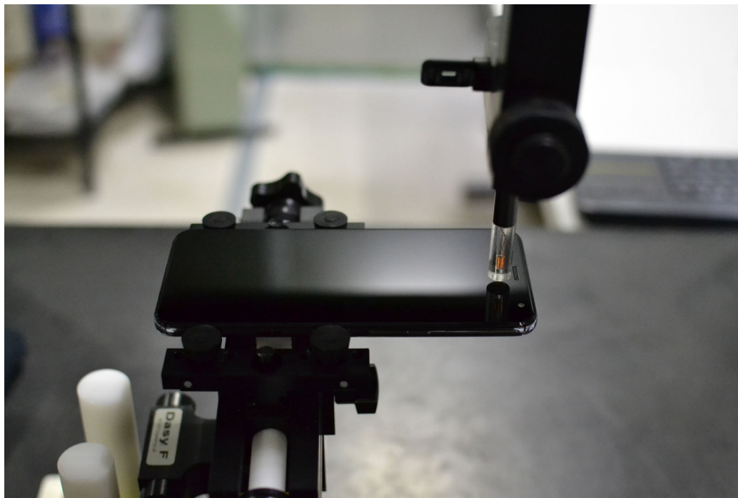
Figure 15-1 Test Setup for Wireless Device
