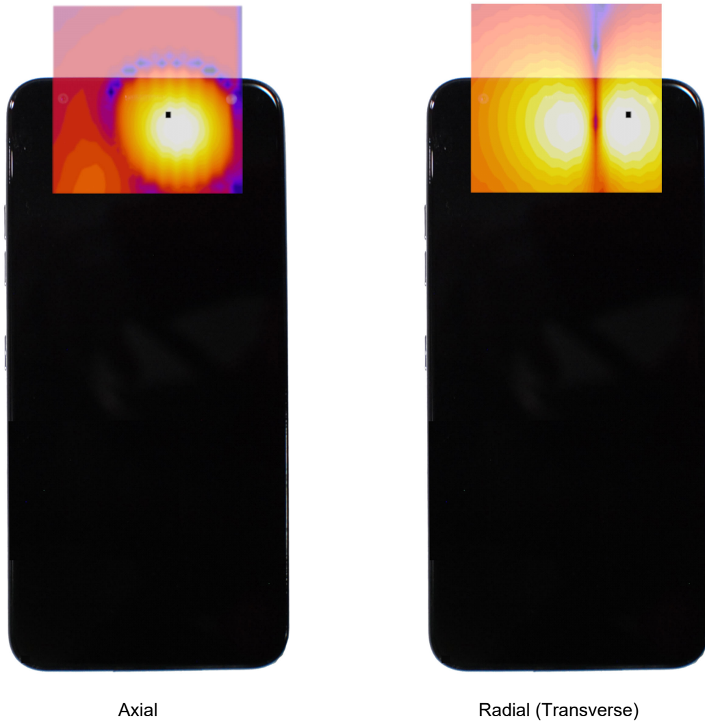
Figure 15-3 CMRS T-Coil Scan Overlay Magnetic Field Distributions
