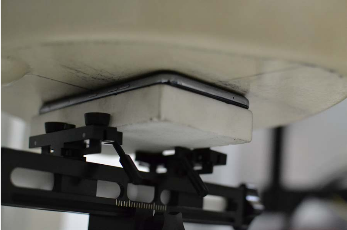
SAR Test Setup Photo 7 – Back Side at 0.0cm
