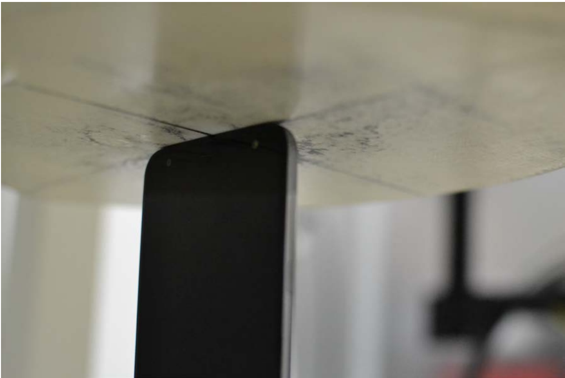
SAR Test Setup Photo 12 – Top Edge at 0.0cm
