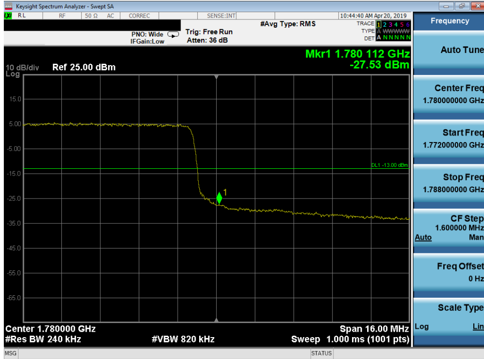
Plot 7-224. Upper Band Edge Plot (Band 66 - 20.0MHz QPSK - Full RB Configuration)
