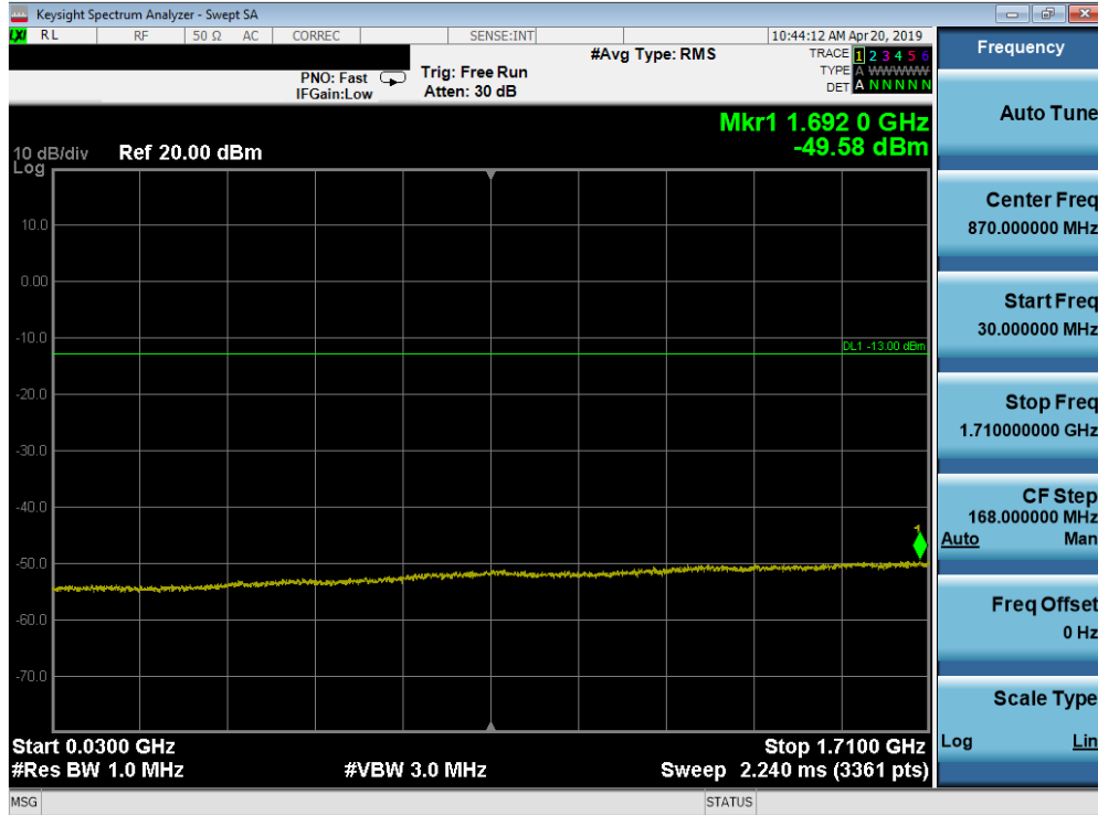
Plot 7-133. Conducted Spurious Plot (Band 66/4 - 20.0MHz QPSK - RB Size 1, RB Offset 0 - High Channel)
