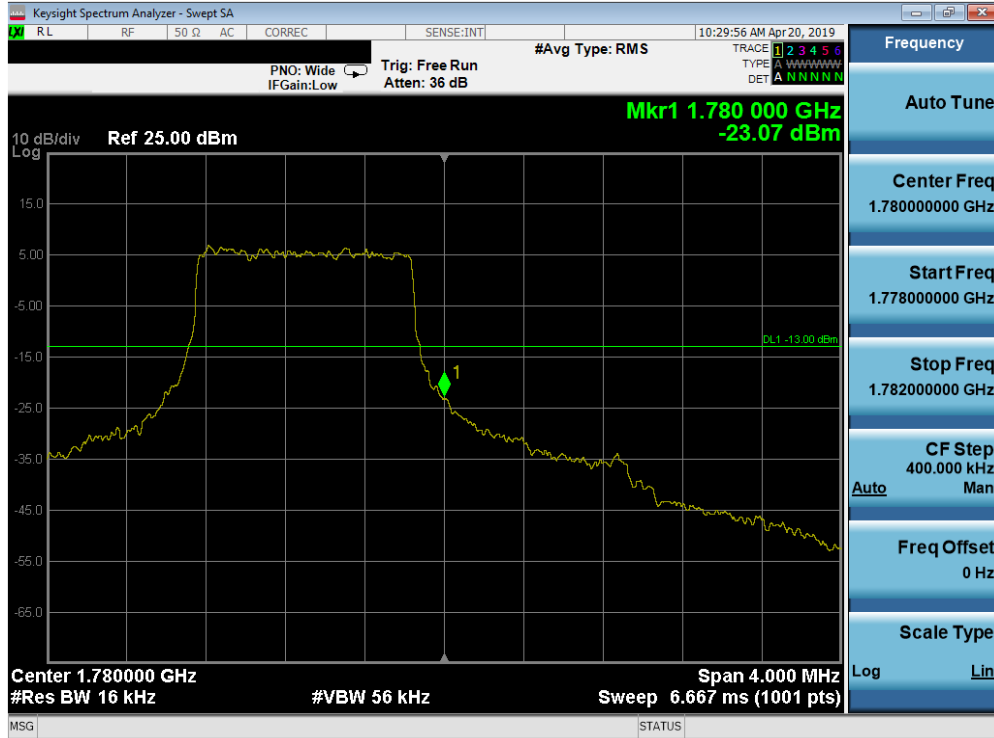
Plot 7-194. Upper Band Edge Plot (Band 66 - 1.4MHz QPSK - Full RB Configuration)
