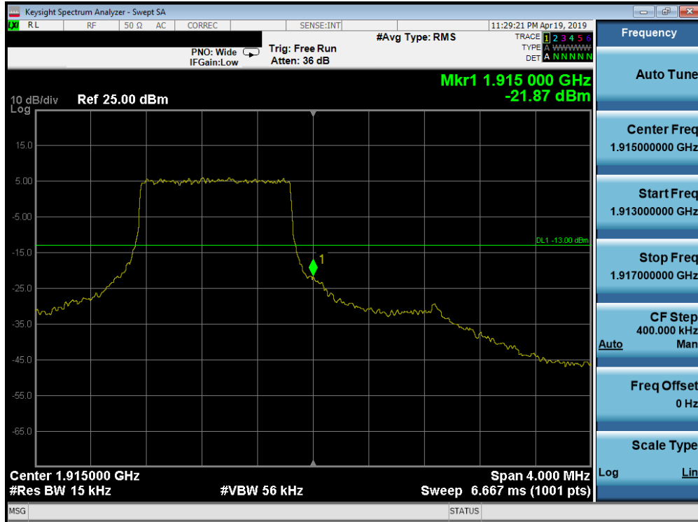
Plot 7-230. Upper Band Edge Plot (Band 25 - 1.4MHz QPSK - Full RB Configuration)
