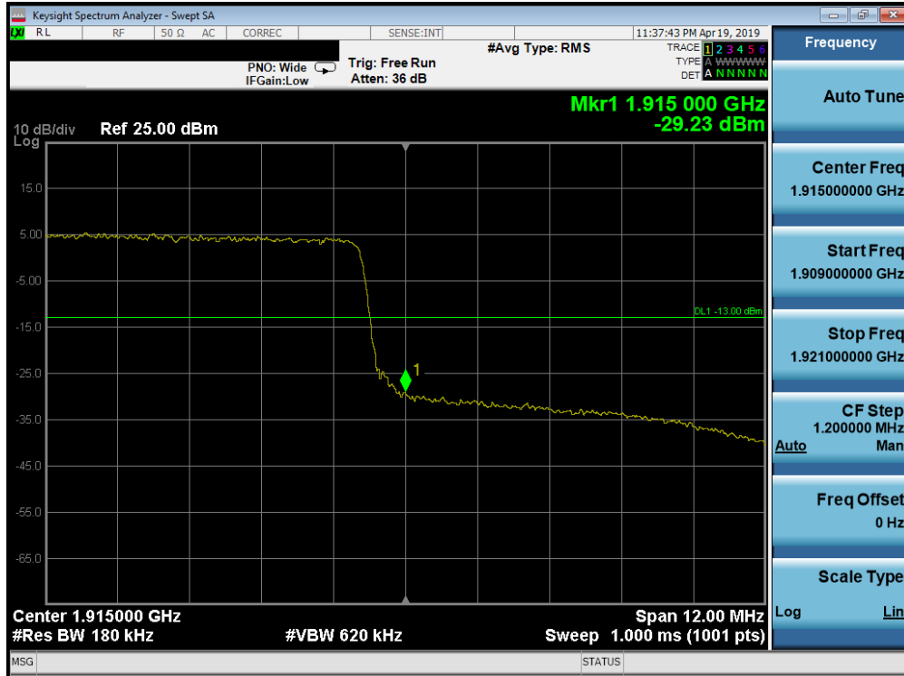
Plot 7-254. Upper Band Edge Plot (Band 25 - 15.0MHz QPSK - Full RB Configuration)
