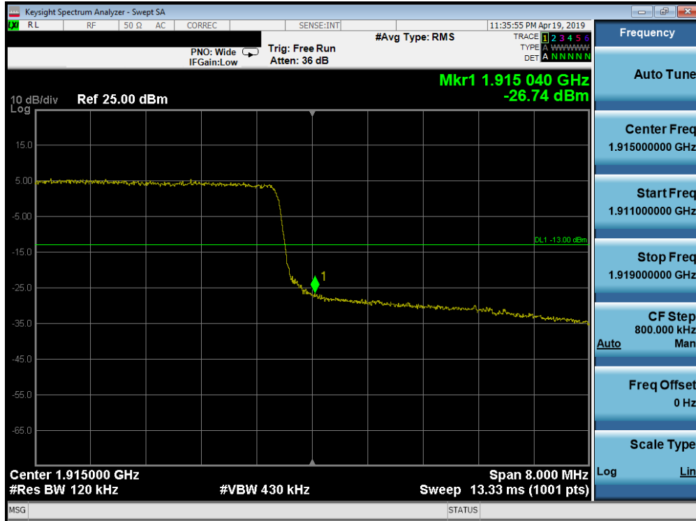
Plot 7-248. Upper Band Edge Plot (Band 25 - 10.0MHz QPSK - Full RB Configuration)
