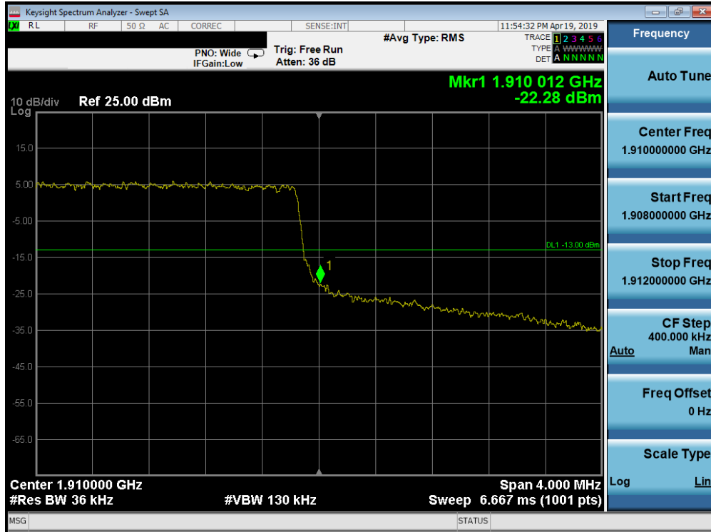
Plot 7-234. Upper Band Edge Plot (Band 2 - 3.0MHz QPSK - Full RB Configuration)
