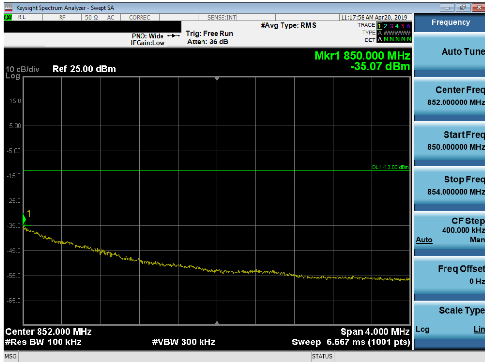
Plot 7-181. Upper Extended Band Edge Plot (Band 26/5 - 1.4MHz QPSK - Full RB Configuration)
