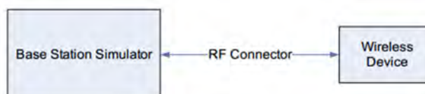
Figure 9.1 Power Measurement Setup
