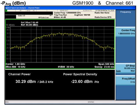
$PAPR (dB) = P_{Pk} (dBm) - P_{Avg} (dBm) = 30.39 dBm - 30.29 dBm = 0.10 dB$
