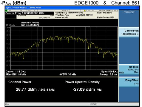
$\overline{PAPR}$  (dB) =  $\overline{P_{Pk}}$  (dBm) -  $\overline{P_{Avg}}$  (dBm) = 30.48 dBm - 26.77 dBm = 3.71 dB
