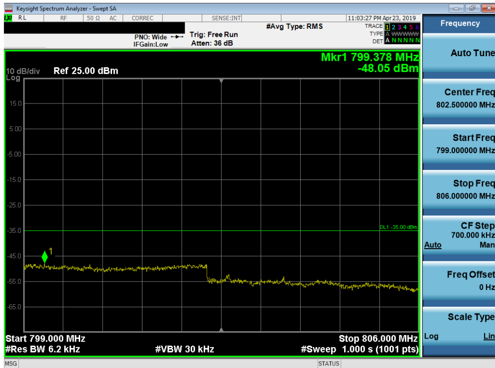
Plot 7-11. Upper Emission Mask Plot (LTE Band 14, 5MHz QPSK – RB Size 25)
