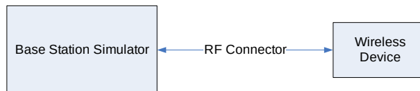
Figure 9-2 Power Measurement Setup
