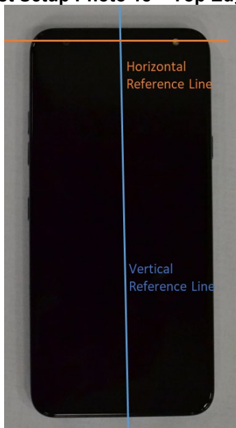
SAR Test Setup Photo 19 – Vertical and Horizontal Reference Lines
