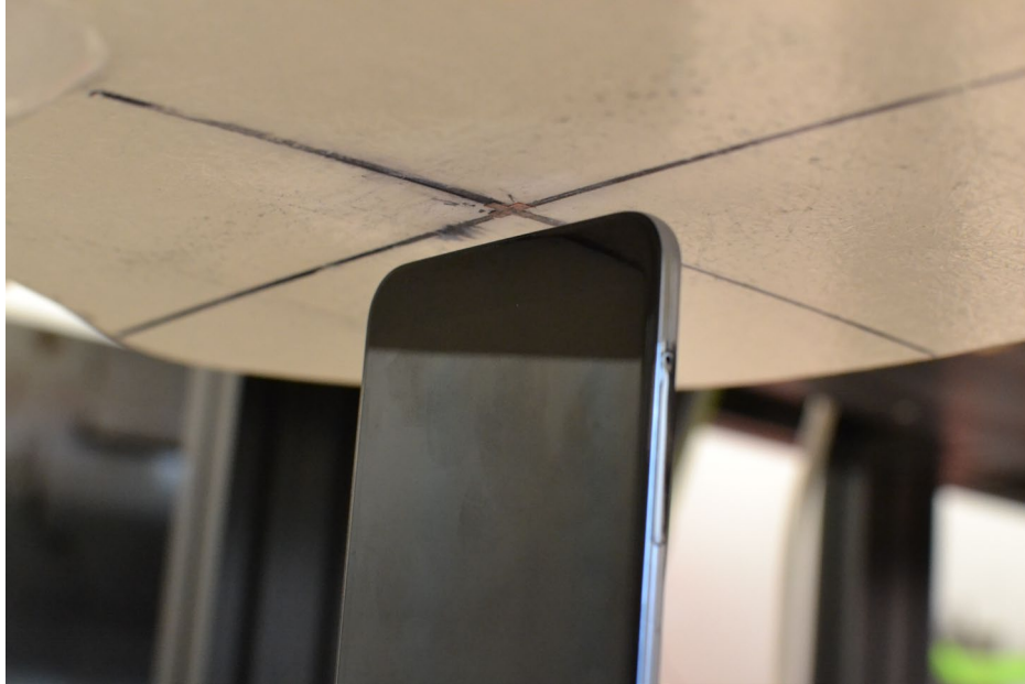
SAR Test Setup Photo 12 – Bottom Edge 4mm
