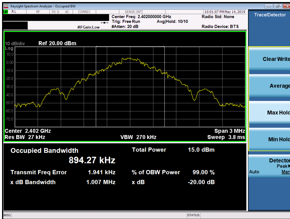
Plot 7-1. 20dB Bandwidth Plot (Bluetooth, 1Mbps – Ch. 0)
