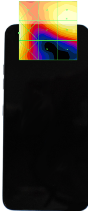
Figure 17-3 5x5 Scan grid above WD
