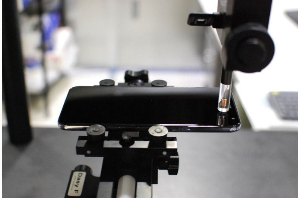
Figure 16-1 Test Setup for Wireless Device
